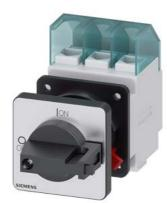
SENTRON, Switch disconnector 3LD, main switch, 3-pole, lu: 32 A, Operating power / at AC-23 A at 400 V: 11.5 kW, front-mounted, knob-operated mechanism, black, central mounting 22.5 mm of the handle
