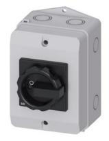
SENTRON, Switch disconnector 3LD, main switch, 3-pole, lu: 32 A, Operating power / at AC-23 A at 400 V: 11.5 kW, molded-plastic encapsulation for inch cable gland, 1 NC, 1 NO, rotary operating mechanism, black
