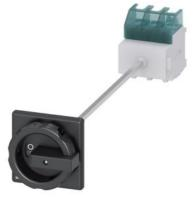
SENTRON, Switch disconnector 3LD, main switch, 3-pole, lu: 63 A, Operating power / at AC-23 A at 400 V: 22 kW, floor mounting with door coupling, rotary operating mechanism, black, 4-hole mounting of the handle
