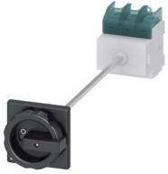
SENTRON, Switch disconnector 3LD, main switch, 3-pole, lu: 100 A, Operating power / at AC-23 A at 400 V: 37 kW, floor mounting with door coupling, rotary operating mechanism, black, 4-hole mounting of the handle
