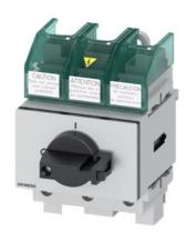
SENTRON, Molded case switch 3LD5 UL, Main switch, 3-pole, certified according to UL489 UL60947-4-1 and IEC60947-3, UL: 60A, SCCR 50kA at 480VAC, Operating power at 480VAC 3-phase: 40hp, IEC: 63A, Operating power at AC-23A at 400V: 30kW, floor mounting with direct handle, black, incl. terminal covers for the infeed side
