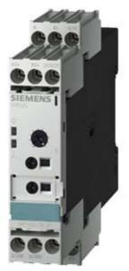
Timing relay, Multifunction Phased-out product !!! For further information, please contact our sales department 2 change-over contacts, 16 functions 15 time ranges (0.05 s-100 h) 24 V, 100-127 V AC and 24 V DC at 50/60 Hz AC with LED, Screw terminal
