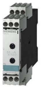
Timing relay, electronic Phased-out product !!! For further information, please contact our sales department with star-delta (wye-delta) function 1...20 s, Overshoot time 30-600 s 0.85 ...1.1 US 24 V AC/DC, 200...240 V AC at 50/60 Hz AC screw terminal
