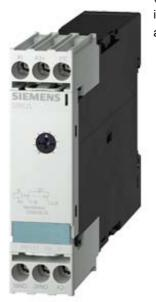
Timing relay, electronic Phased-out product !!! For further information, please contact our sales department with star-delta (wye-delta) function 1 NO contact, delayed 1 NO contact, instantaneous 1 time range 1...20 s 24 V AC/DC and 200...240 V AC at 50/60 Hz AC screw terminal
