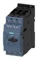
Circuit breaker size S2 for motor protection, CLASS 10 A-release 35...45 A N-release 650 A screw terminal Standard switching capacity with transverse auxiliary switches 1 NO+1 NC
