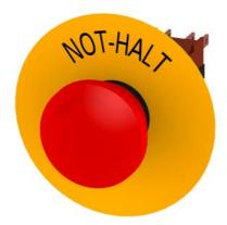
Emergency stop mushroom pushbutton, 16 mm, round, plastic, red, latching, with rotate-to-unlatch mechanism, according to ISO 13850, 1 NC, with yellow backing plate, EMERGENCY STOP
