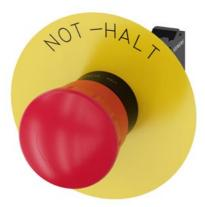
EMERGENCY STOP mushroom-type actuator, 22 mm, round, plastic, red, 40 mm, positive latching, according to EN ISO 13850, rotate-to-unlatch, with yellow backing plate, inscription: NOT-HALT, with holder, 1 NC, spring-type terminal
