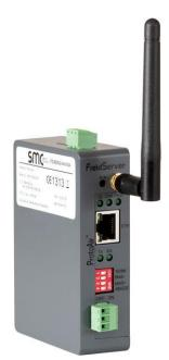
The BACnet Explorer NG offers access anywhere through its own Wi-Fi access point. Meaning connection to your devices is available directly from the Explorer or through the cloud with SMC Cloud.
