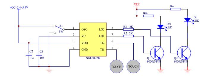
Note: The touching sensitivity could be regulated by modifying the value of C3 (the sampling capacitor between VC and GND). when the difference practical medium material and medium in the form,
