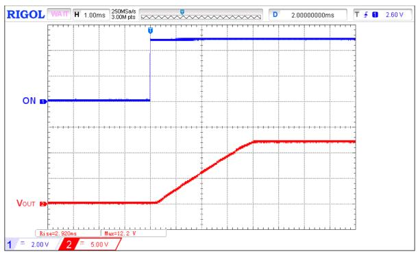
Figure 2. Typical Turn ON operation waveform for V<sub>IN</sub> = 12 V,  $C_{SLEW}$  = 10 nF,  $C_{LOAD}$  = 10  $\mu$ F,  $R_{LOAD}$  = 100  $\Omega$
