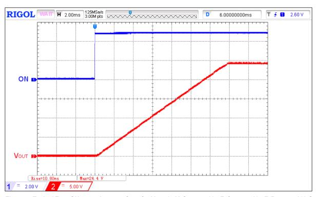
Figure 5. Typical Turn ON operation waveform for  $V_{IN}$  = 24 V,  $C_{SLEW}$  = 18 nF,  $C_{LOAD}$  = 10  $\mu$ F,  $R_{LOAD}$  = 100  $\Omega$  Typical Turn-off Waveforms
