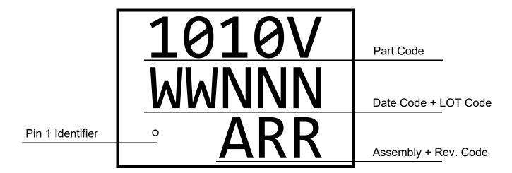
1010V - Part ID Field WW - Date Code Field<sup>1</sup> NNN - Lot Traceability Code Field<sup>1</sup> A - Assembly Site Code Field<sup>2</sup> RR - Part Revision Code Field<sup>2</sup>
