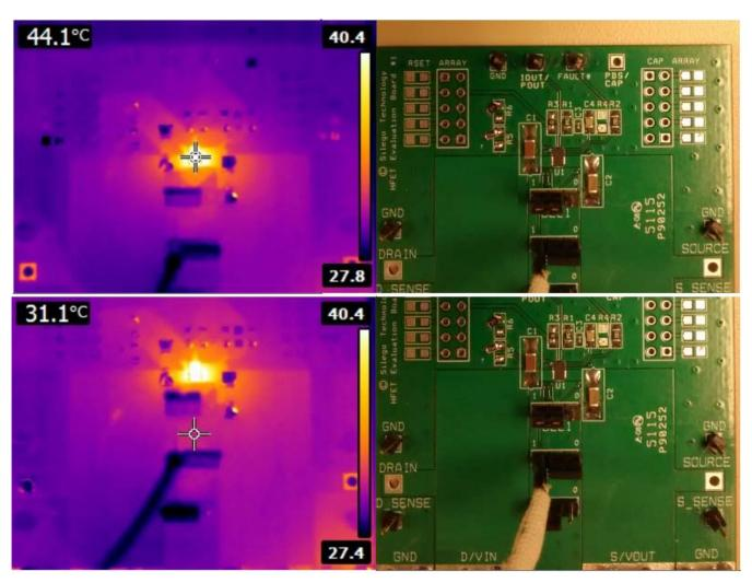
Figure 17. Thermal distribution for  $V_{\rm IN}$  = 24 V,  $I_{\rm DS}$  = 4.5 A after 2 min power up
