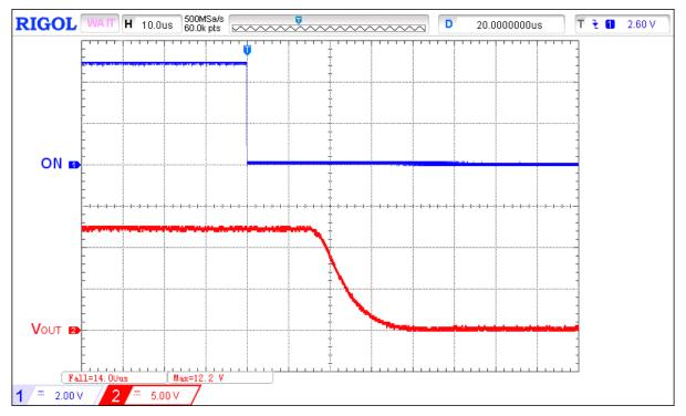
Figure 6. Typical Turn OFF operation waveform for V<sub>IN</sub> = 12 V, C<sub>SLEW</sub> = 10 nF, no C<sub>LOAD</sub> , R<sub>LOAD</sub> = 100  $\Omega$
