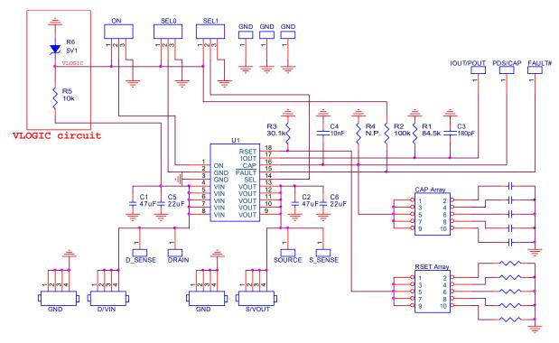
Figure 15. SLG59H1010V Evaluation Board Connection Circuit
