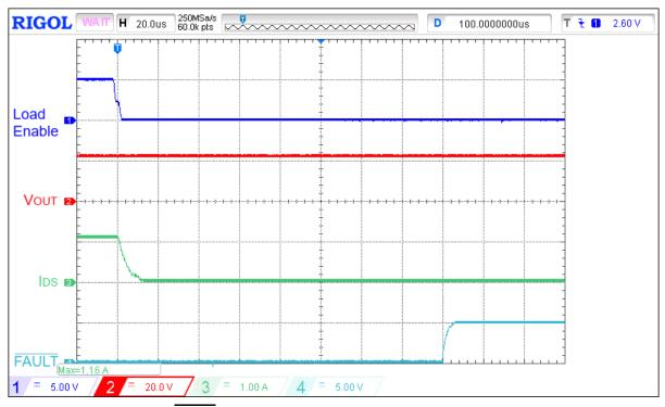
Figure 13. Typical FAULT de-assertion waveform for  $V_{IN}$  = 24 V,  $C_{LOAD}$  = 10  $\mu$ F,  $I_{ACL}$  = 1 A,  $R_{SET}$  = 91 k $\Omega$ , switch out 18.5  $\Omega$  load
