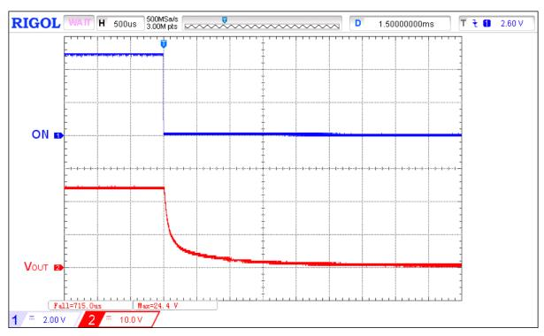
Figure 9. Typical Turn OFF operation waveform for  $V_{IN}$  = 24 V,  $C_{SLEW}$  = 10 nF,  $C_{LOAD}$  = 10  $\mu$ F,  $R_{LOAD}$  = 100  $\Omega$  Typical ACL Operation Waveforms
