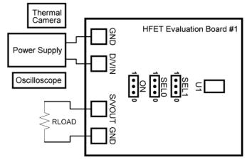
Figure 16. SLG59H1010V Evaluation Board Connection Circuit
