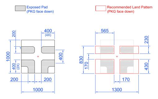
Note: All dimensions shown in micrometers (µm)
