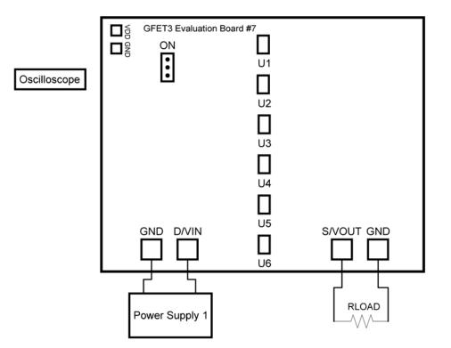
Figure 3. SLG59M1558V Evaluation Board Connection Circuit
