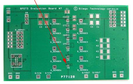
Figure 1. SLG59M1558V Evaluation Board
