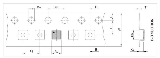
Note: 1.Orientation in carrier: Pin1 is at upper left corner (Quadrant 1).
