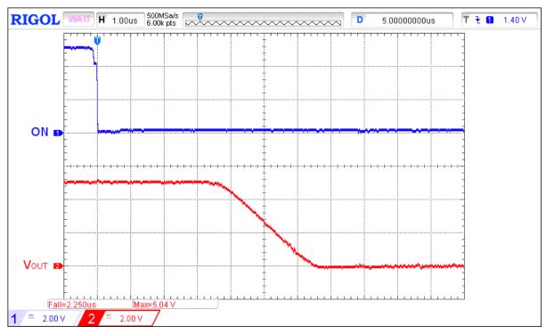
Figure 5. Typical Turn OFF operation waveform for V<sub>IN</sub> = 5 V, no  $C_{LOAD}$  ,  $R_{LOAD}$  = 10  $\Omega$
