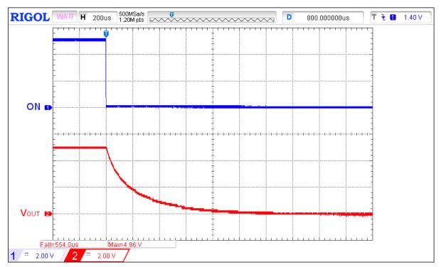
Figure 6. Typical Turn OFF operation waveform for  $V_{IN}$  = 5 V,  $C_{LOAD}$  = 30  $\mu$ F,  $R_{LOAD}$  = 10  $\Omega$
