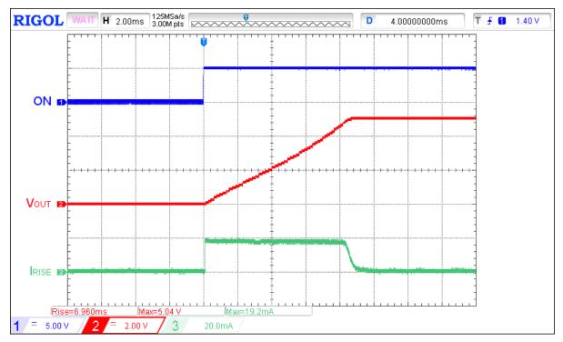
Figure 2. Typical Turn ON operation waveform for  $V_{IN}$  = 5 V,  $C_{LOAD}$  = 30  $\mu F$
