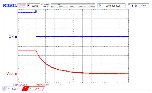
Figure 4. Typical Turn OFF operation waveform for V<sub>IN</sub> = 2.5 V,  $C_{LOAD}$  = 30  $\mu$ F,  $R_{LOAD}$  = 10  $\Omega$
