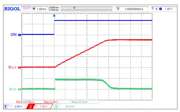
Figure 1. Typical Turn ON operation waveform for  $V_{IN}$  = 2.5 V,  $C_{LOAD}$  = 30  $\mu F$
