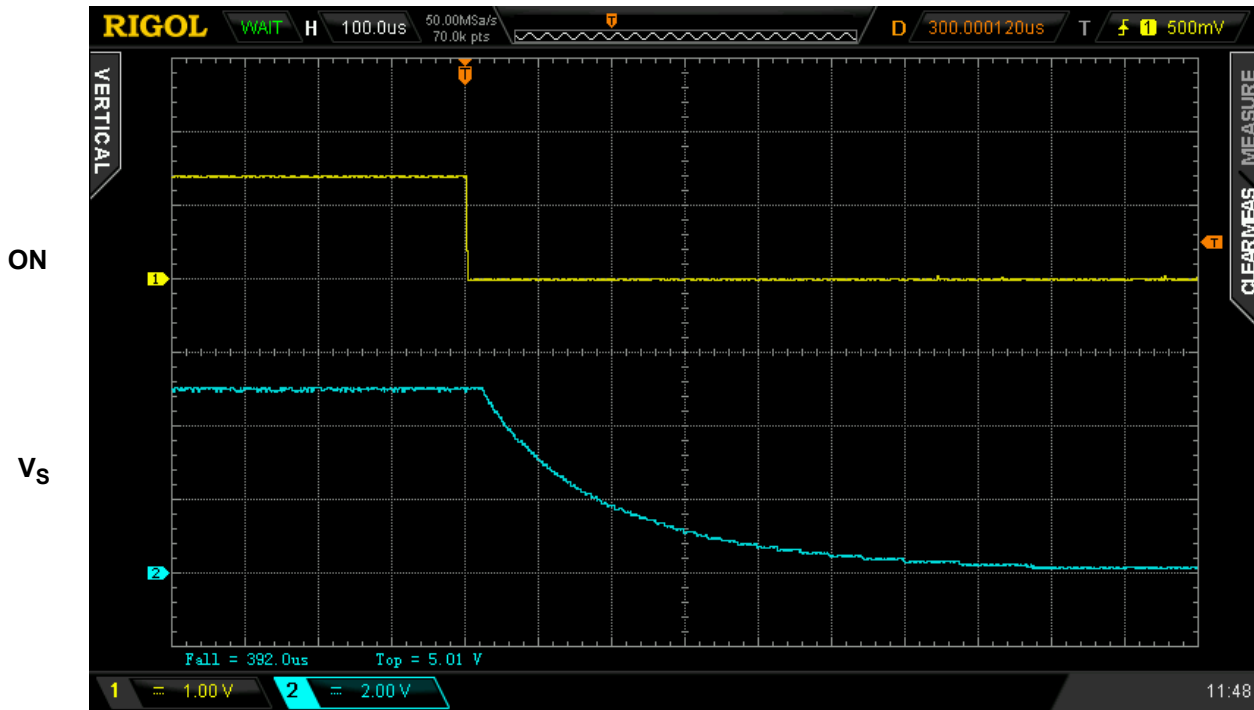
Figure 4. Typical Turn OFF operation waveform for V_{DD} = V_D = 5\text{ V} , C_{SLEW} = 4\text{ nF} , C_{LOAD} = 10\ \mu\text{F} , R_{LOAD} = 20\ \Omega
