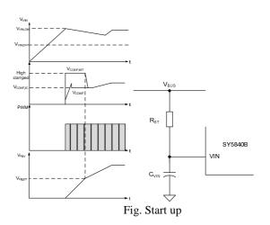
This operation is aimed to build up enough output voltage for auxiliary winding bias supply as quickly as possible. It is enabled only one time just when  $V_{VIN}$  is over  $V_{VIN,ON}$ .
