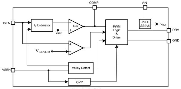
Figure3. Block Diagram
