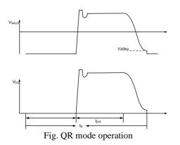
The voltage across drain and source of the primary MOSFET is reflected by the auxiliary winding of the Flyback transformer. VSEN pin detects the voltage across the auxiliary winding by a resistor divider. When the voltage across drain and source of the primary MOSFET is at voltage valley, the MOSFET would be turned on.
