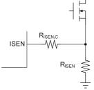
Fig. feed-forward resistor
