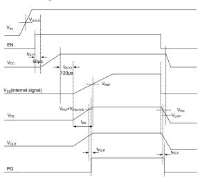
After the input voltage exceeds its own UVLO (rising) threshold,  $V_{CC}$  is turned on after EN is enabled for one delay time  $t_{DLY1}$ , the buck regulator is turned on after another delay time  $t_{DLY2}$  after VCC voltage is set up. When the output voltage is 90% of the regulation point, PG becomes high-impedance after one delay time  $t_{PG,R}$ .
