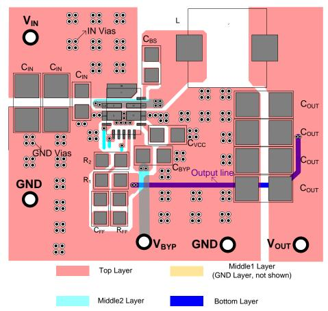
Figure 4. PCB Layout Suggestion
