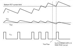
The device supports programmable valley current limit threshold. Pull ILMT pin low, floating or high for 3 gears successively increasing valley current limit threshold. When the valley current limit occurs, the output current limit value is
