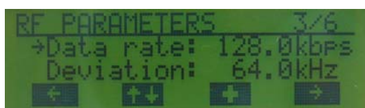
Figure 8. Menu Page: RF Parameters 3/6 (Modulation is 2GFSK)
