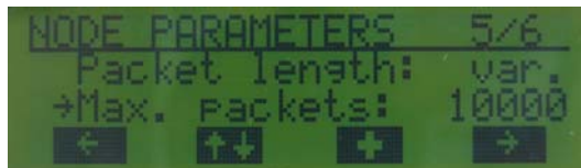
Figure 12. Menu Page: Node Parameters 5/6 (Rx mode)
