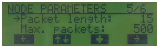
Figure 11. Menu Page: Node Parameters 5/6 (Tx/TRx mode)
