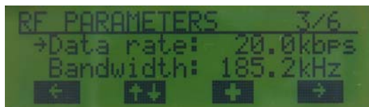
Figure 9. Menu Page: RF Parameters 3/6 (Modulation is OOK)
