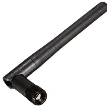
4" Antenna with Hinged SMA Reverse Polarity Plug for 2.4/5 GHz
