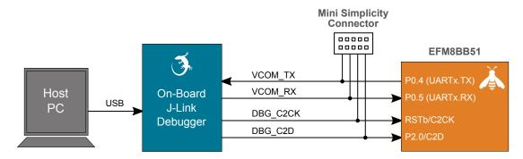
Figure 3.4. On-Board Debugger Connections
