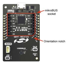
Figure 3.6. mikroBUS Add-on Board Orientation
