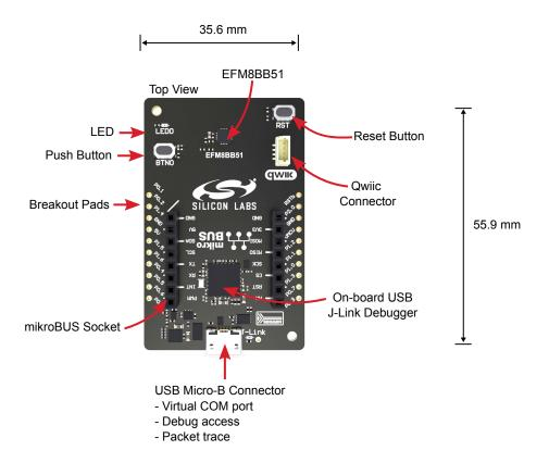
Figure 1.1. BB51 Explorer Kit Hardware Layout
