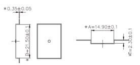
Figure 10.2. Dimensions of the Module Slot on Tape
