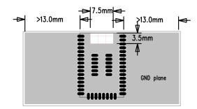
Figure 5.1. Recommended Application PCB Layout for WGM110A Module
