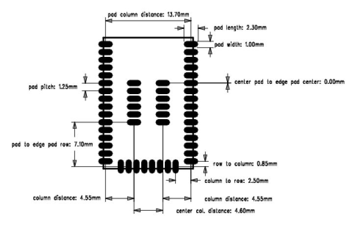
Figure 8.5. Recommended Application PCB Land Pattern
