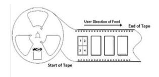
Figure 10.6. Module Orientation in Tape
