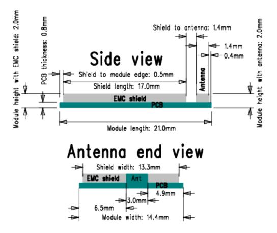
Figure 8.2. Side and Antenna End View Dimensions (WGM110A)
