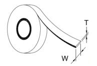
Figure 10.3. Dimensions of the Cover Tape
