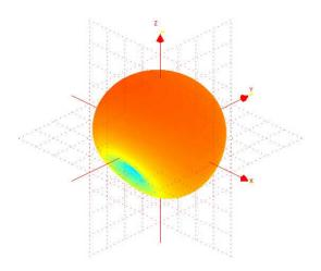
Figure 7.1. Typical 3D Radiation Pattern for WGM110A Module
