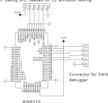
RF debug SPI, needed for CE emission testing
