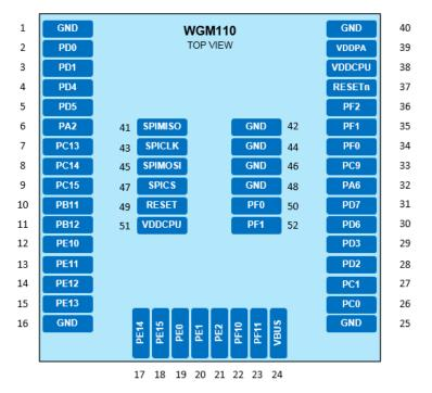
Figure 2.1. WGM110 Pinout (Top View)
