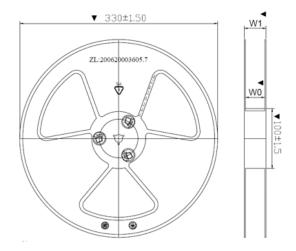
Figure 10.4. Reel Dimensions - Side View
