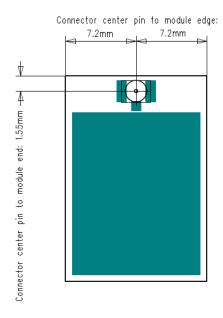
Figure 8.4. u.FL Connector Placement on the WGM110E Module
