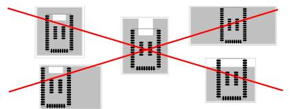
Figure 5.2. Non-optimal Application PCB Layouts for WGM110A Module
