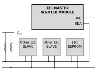
Figure 3.5. WGM110 Acting as an I<sup>2</sup>C Master with Several I2C Slaves Connected to the Module
