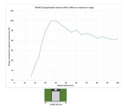
Figure 5.3. Guideline For the Achievable Range vs. Ground Plane Width for WGM110A
