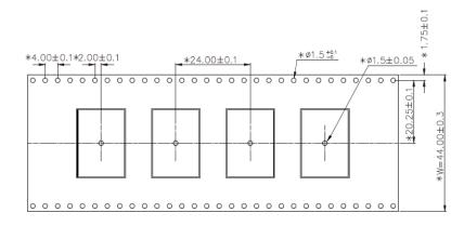
Figure 10.1. Tape Dimensions - Top View
