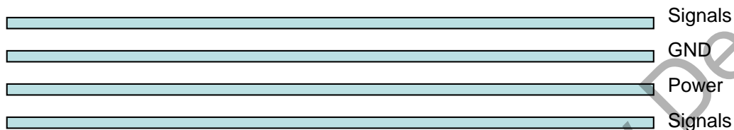
Figure 21: Typical 4-layer PCB construction
