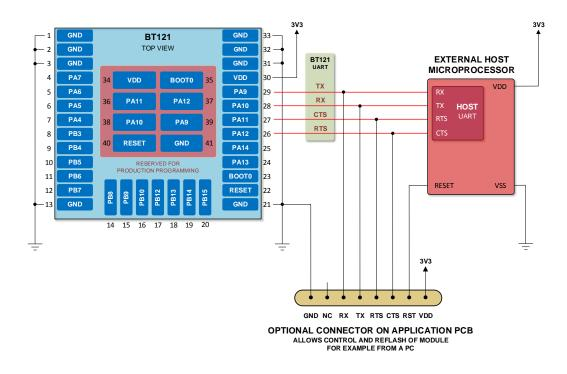
Figure 18 Connecting an external host with BT121 using UART
