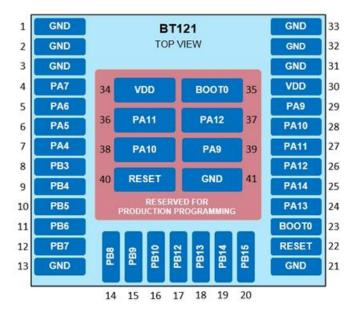
Figure 4 BT121 pin-out (top view)
