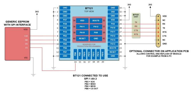
Figure 19 Connecting an external device with BT121 using SPI interface
