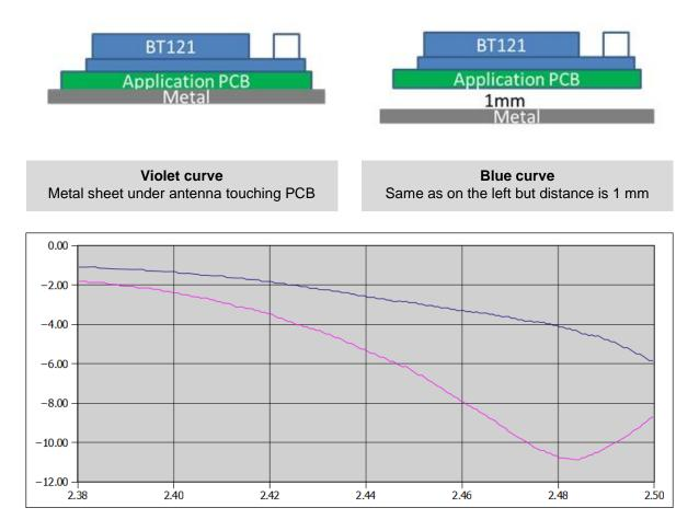
Figure 9 Effect of a metal sheet placed under the antenna on antenna matching
