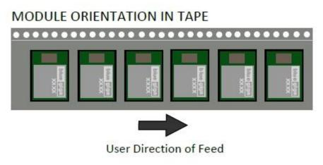
Figure 25 Module orientation in tape and feed direction
