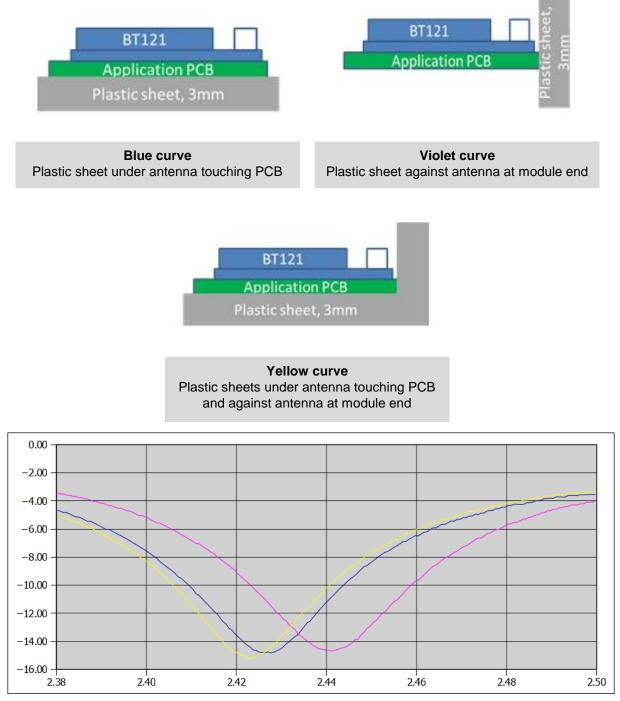
Figure 8 Proximity effect of a 3 mm plastic sheet on antenna matching with different placements
