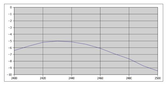
Figure 11 Antenna efficiency related to frequency
