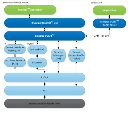
Figure 17 Bluegiga Bluetooth Smart Ready software stack
