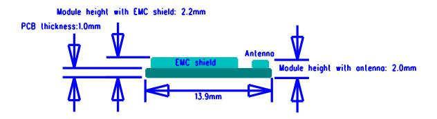
Figure 23 BT121 module side view dimensions
