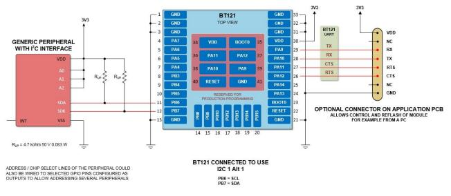
Figure 20 Connecting to an I2C peripheral
