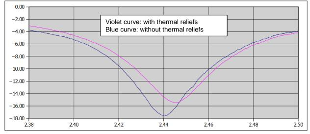
Figure 7 Typical antenna matching
