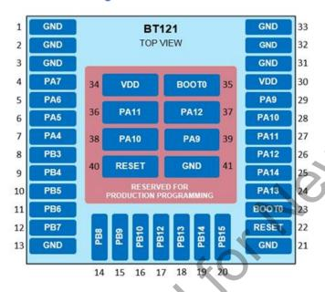
Figure 4 BT121 pin-out (top view)
