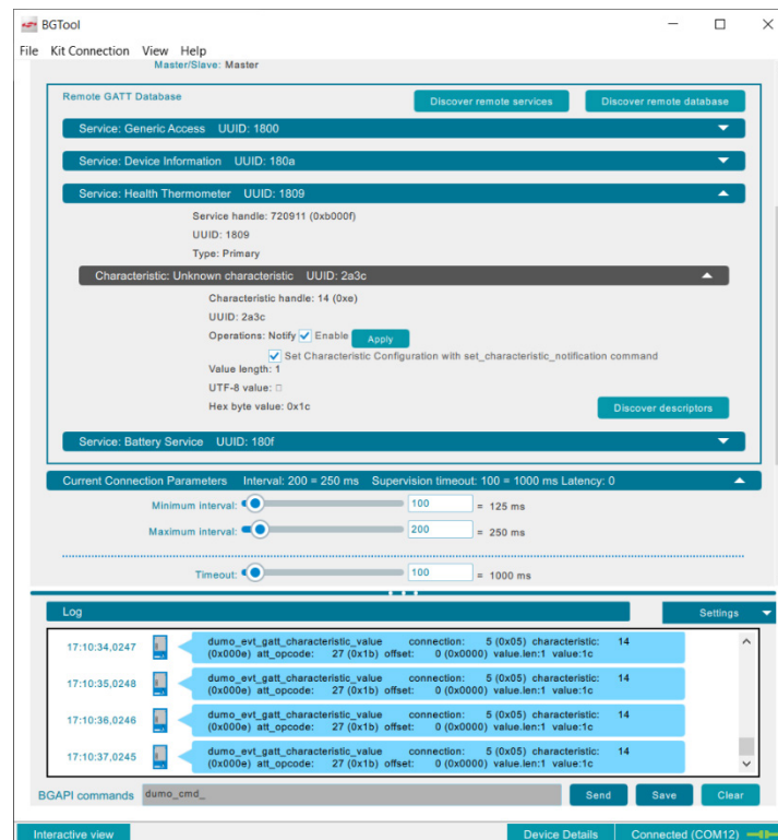
Figure 6.10 Health Thermometer Characteristics Updating with Notifications
