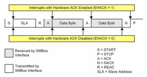
Figure 21.6. Typical Master Read Sequence
