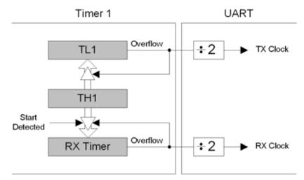
Figure 22.2. UART0 Baud Rate Logic
