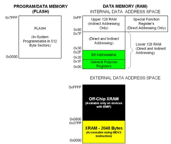
Figure 13.2. On-Chip Memory Map for 32 kB Devices (C8051F38A/B)
