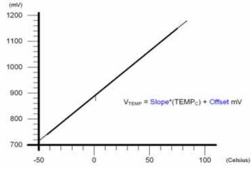
Figure 6.2. Typical Temperature Sensor Transfer Function
