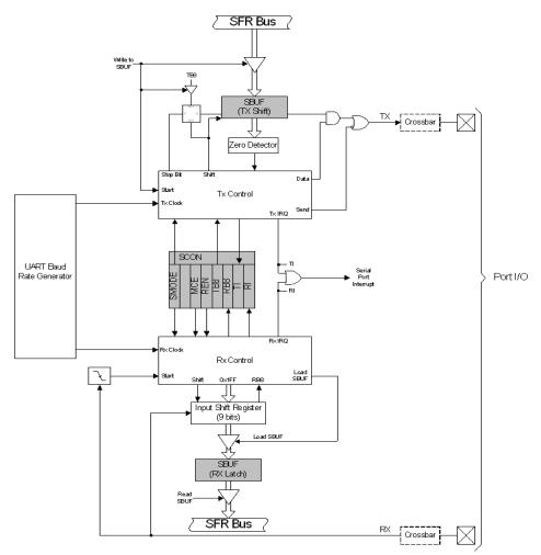
Figure 22.1. UART0 Block Diagram
