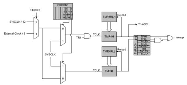
Figure 25.13. Timer 4 8-Bit Mode Block Diagram
