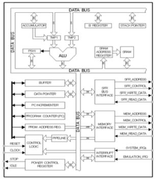
Figure 11.1. CIP-51 Block Diagram
