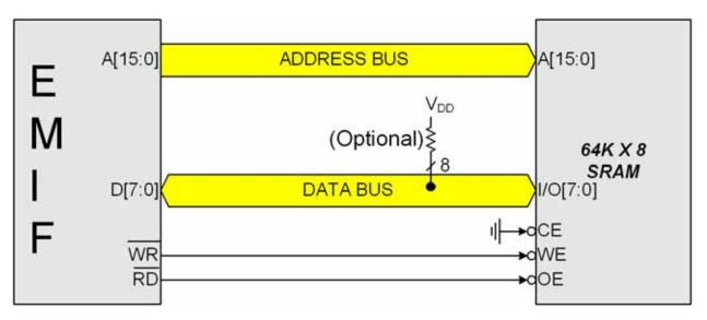
Figure 14.2. Non-multiplexed Configuration Example
