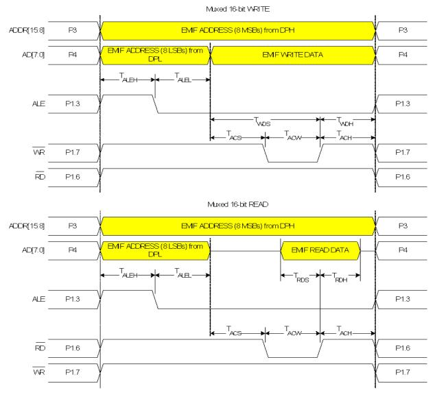
Figure 14.7. Multiplexed 16-bit MOVX Timing
