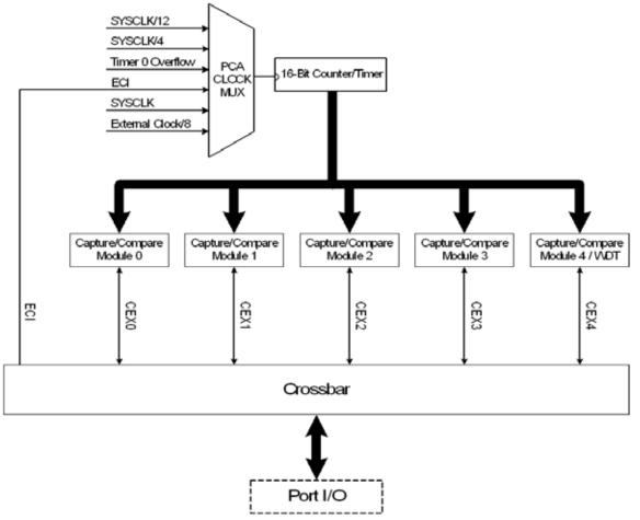
Figure 26.1. PCA Block Diagram
