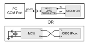
Figure 23.5. Typical UART Interconnect Diagram
