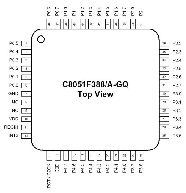
Figure 3.1. TQFP-48 (C8051F388/A) Pinout Diagram (Top View)
