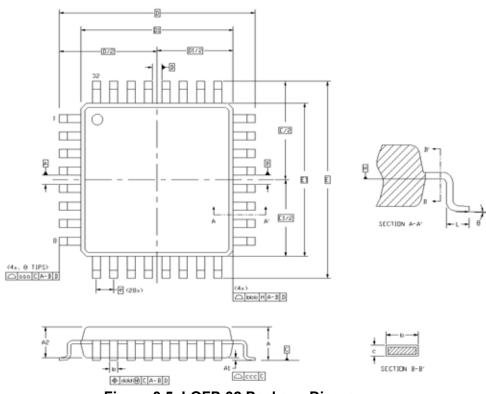
Figure 3.5. LQFP-32 Package Diagram
