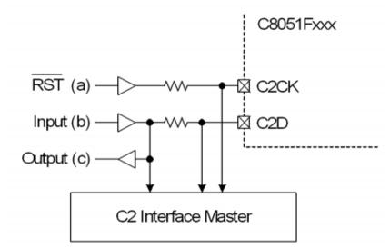
Figure 27.1. Typical C2 Pin Sharing
