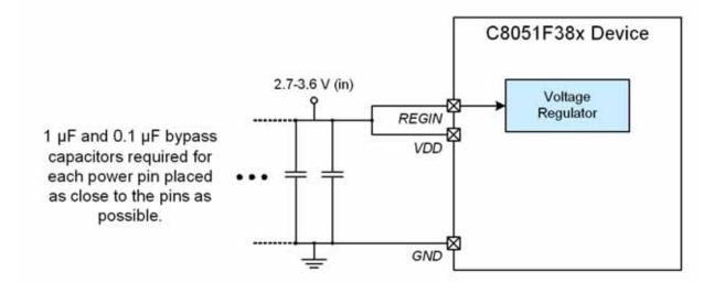
Figure 4.2. Connection Diagram with Voltage Regulator Not Used
