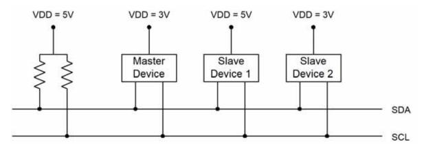
Figure 21.2. Typical SMBus Configuration
