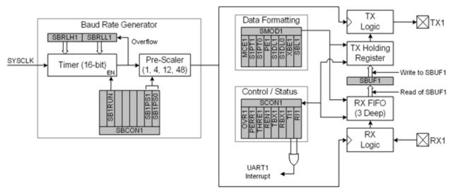
Figure 23.1. UART1 Block Diagram
