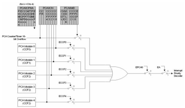
Figure 26.3. PCA Interrupt Block Diagram
