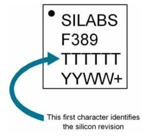
Figure 28.3. Device Package – QFN32
