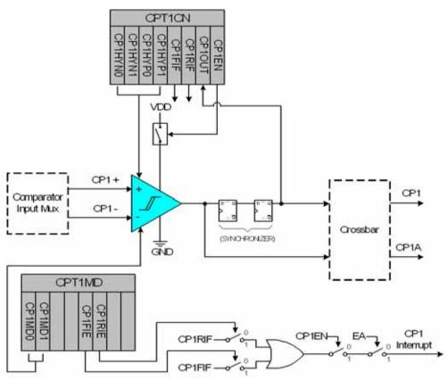
Figure 8.2. Comparator1 Functional Block Diagram
