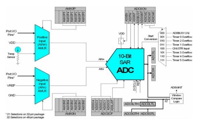
Figure 6.1. ADC0 Functional Block Diagram
