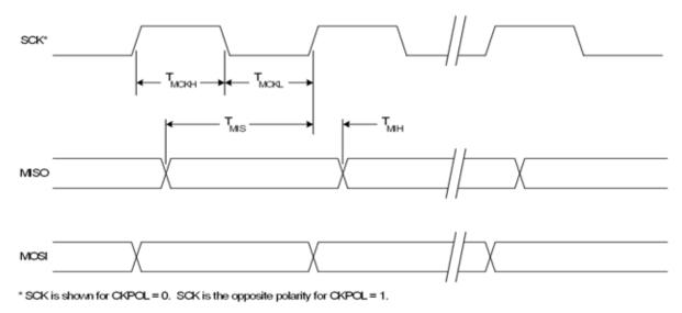
Figure 24.9. SPI Master Timing (CKPHA = 1)
