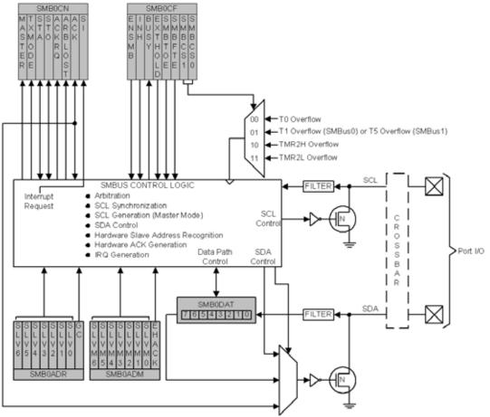
Figure 21.1. SMBus Block Diagram
