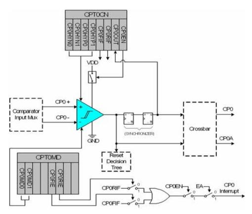
Figure 8.1. Comparator0 Functional Block Diagram
