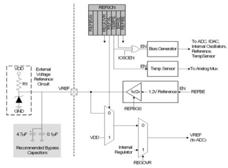
Figure 7.1. Voltage Reference Functional Block Diagram
