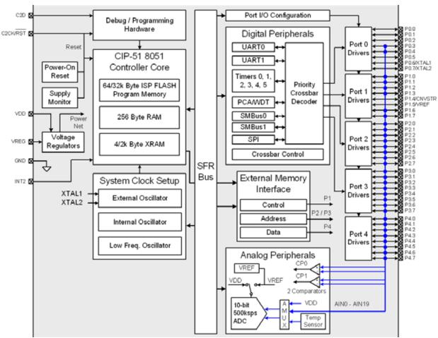
Figure 1.1. C8051F388/A Block Diagram
