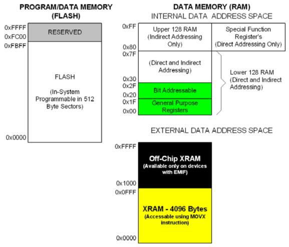
Figure 13.1. On-Chip Memory Map for 64 kB Devices (C8051F388/9)
