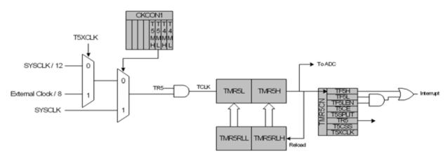
Figure 25.14. Timer 5 16-Bit Mode Block Diagram
