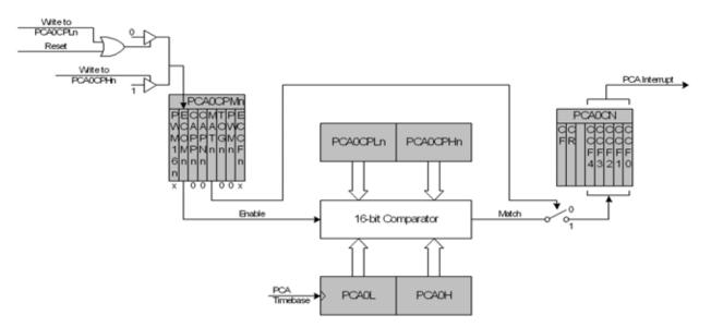
Figure 26.5. PCA Software Timer Mode Diagram
