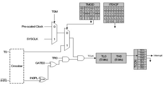
Figure 25.1. T0 Mode 0 Block Diagram
