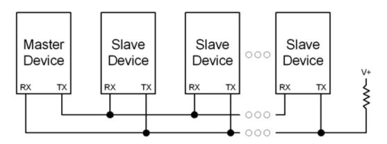
Figure 22.6. UART Multi-Processor Mode Interconnect Diagram
