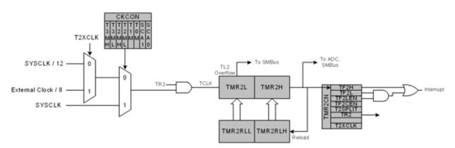
Figure 25.4. Timer 2 16-Bit Mode Block Diagram
