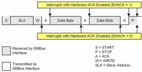
Figure 21.7. Typical Slave Write Sequence
