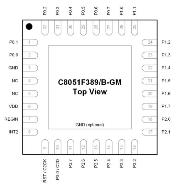
Figure 3.7. QFN-32 (C8051F389/B) Pinout Diagram (Top View)
