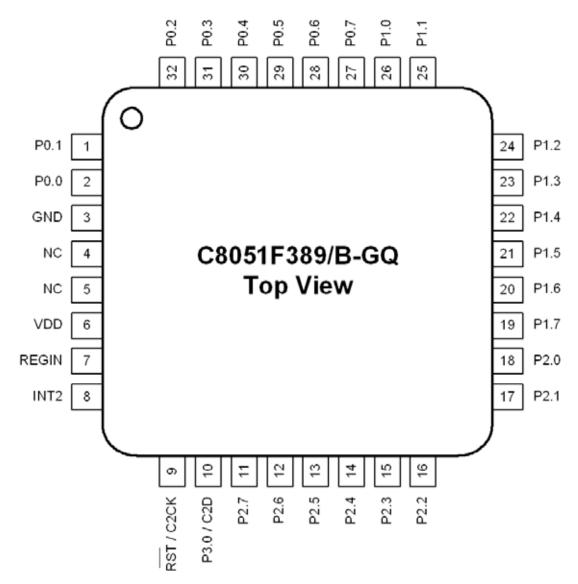
Figure 3.4. LQFP-32 (C8051F389/B) Pinout Diagram (Top View)
