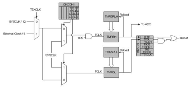
Figure 25.15. Timer 5 8-Bit Mode Block Diagram
