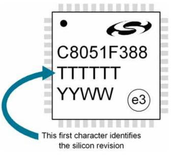
Figure 28.1. Device Package – TQFP48
