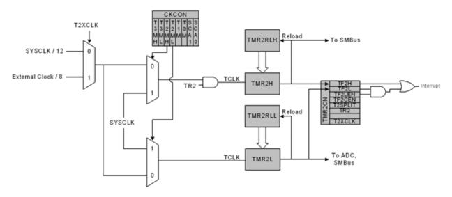
Figure 25.5. Timer 2 8-Bit Mode Block Diagram
