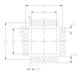
Figure 3.9. QFN-32 Recommended PCB Land Pattern
