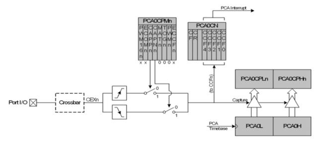
Figure 26.4. PCA Capture Mode Diagram
