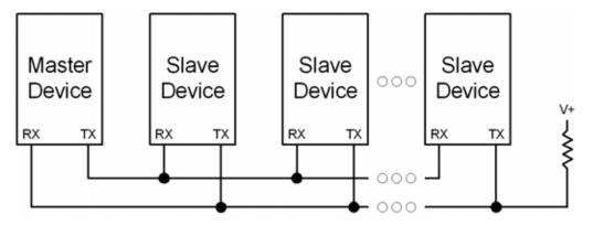
Figure 23.6. UART Multi-Processor Mode Interconnect Diagram
