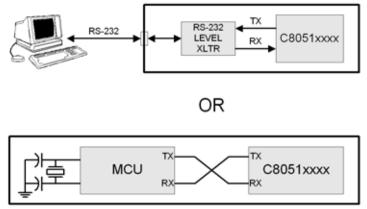
Figure 22.3. UART Interconnect Diagram
