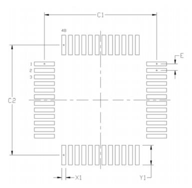
Figure 3.3. TQFP-48 Recommended PCB Land Pattern
