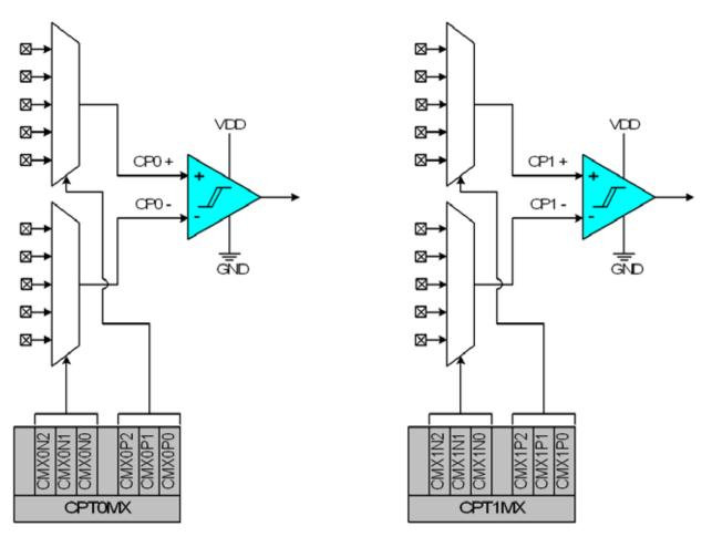
Figure 8.4. Comparator Input Multiplexer Block Diagram
