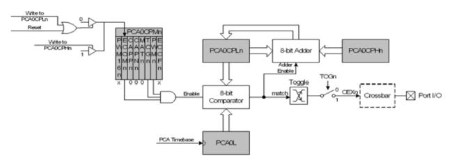
Figure 26.7. PCA Frequency Output Mode
