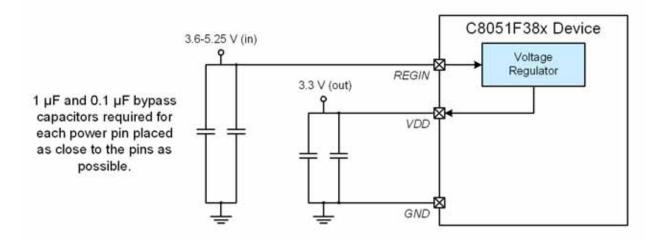
Figure 4.1. Connection Diagram with Voltage Regulator Used
