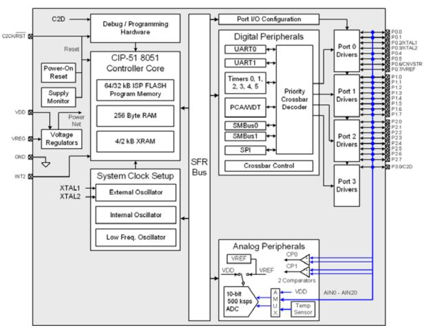
Figure 1.2. C8051F389/B Block Diagram
