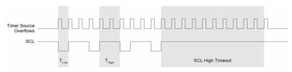
Figure 21.4. Typical SMBus SCL Generation
