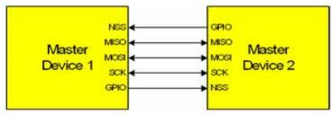
Figure 24.2. Multiple-Master Mode Connection Diagram
