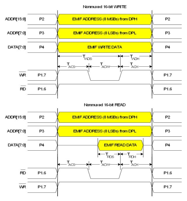
Figure 14.4. Non-Multiplexed 16-bit MOVX Timing
