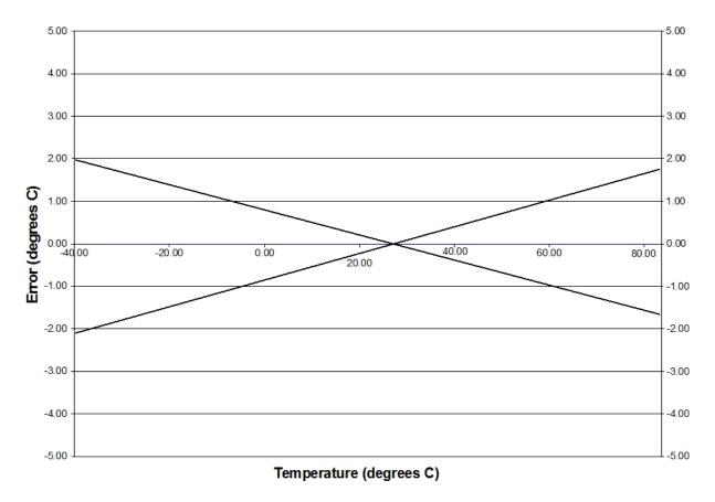
Figure 6.3. Temperature Sensor Error with 1-Point Calibration
