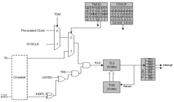
Figure 25.2. T0 Mode 2 Block Diagram
