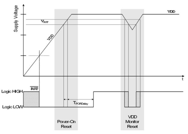
Figure 17.2. Power-On and V<sub>DD</sub> Monitor Reset Timing
