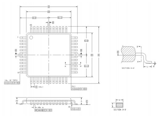
Figure 3.2. TQFP-48 Package Diagram
