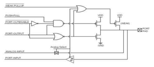
Figure 20.2. Port I/O Cell Block Diagram
