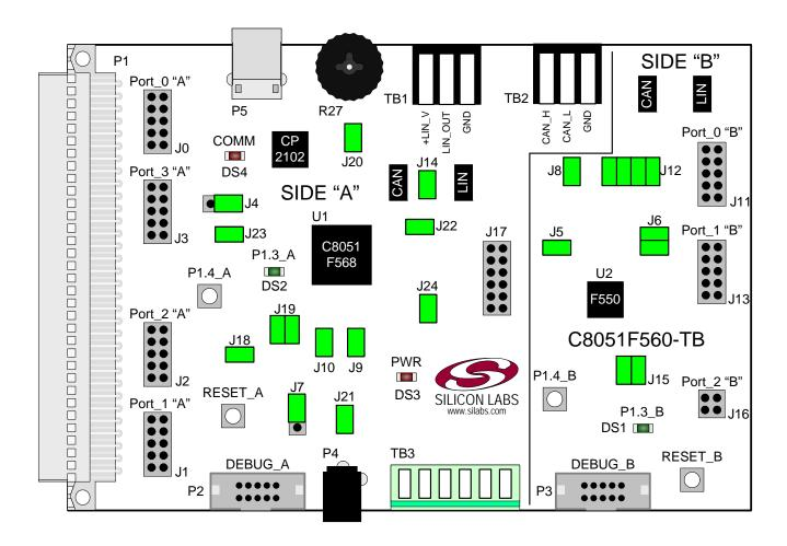
Figure 5. C8051F560 Target Board Shorting Blocks: Factory Defaults
