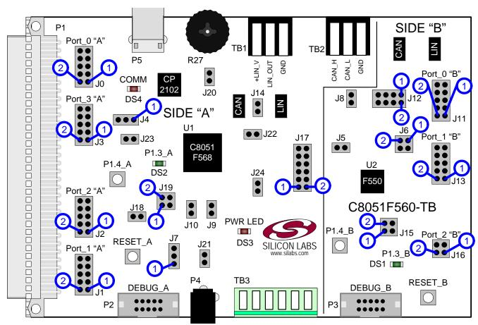
Figure 4. C8051F560 Target Board with Pin Numbers
