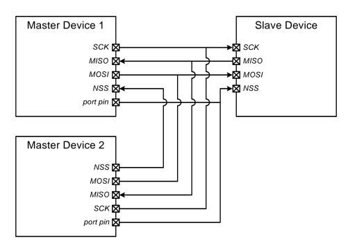
Figure 23.2. Multiple-Master Mode Connection Diagram
