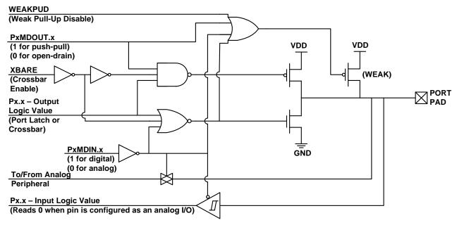
Figure 21.4. Port I/O Cell Block Diagram
