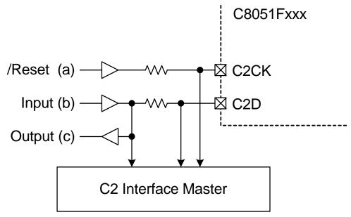
Figure 29.1. Typical C2 Pin Sharing
