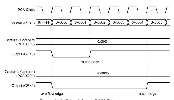
Figure 20.6. Edge-Aligned PWM Timing
