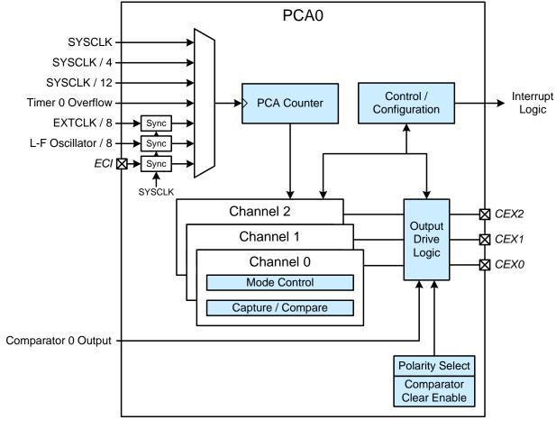
Figure 20.1. PCA0 Block Diagram
