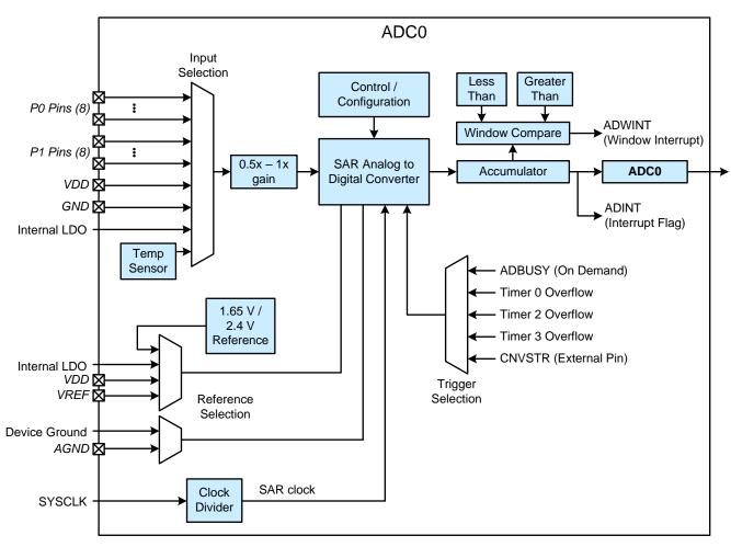
Figure 14.1. ADC0 Functional Block Diagram
