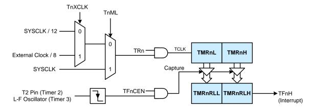
Figure 25.6. Capture Mode Block Diagram
