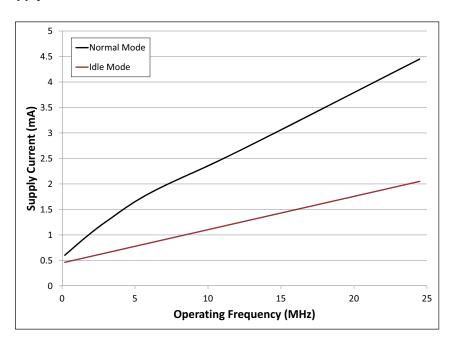
Figure 1.1. Typical Operating Current Running From 24.5 MHz Internal Oscillator
