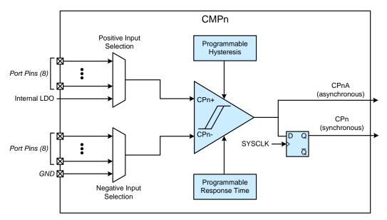
Figure 17.1. Comparator Functional Block Diagram
