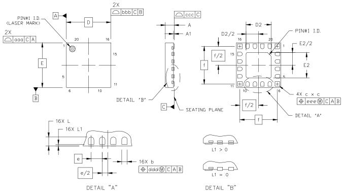
Figure 6.1. QFN-20 Package Drawing
