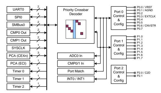
Figure 21.1. Port I/O Functional Block Diagram
