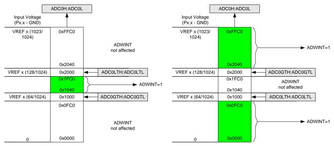
Figure 14.7. ADC Window Compare Example: Left-Justified Single-Ended Data
