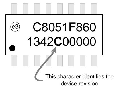
Figure 28.3. SOIC-16 Package Revision Marking
