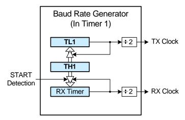
Figure 26.2. UARTO Baud Rate Logic
