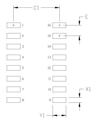
Figure 7.2. SOIC-16 PCB Land Pattern
