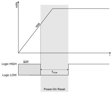
Figure 22.2. Power-on Reset Timing
