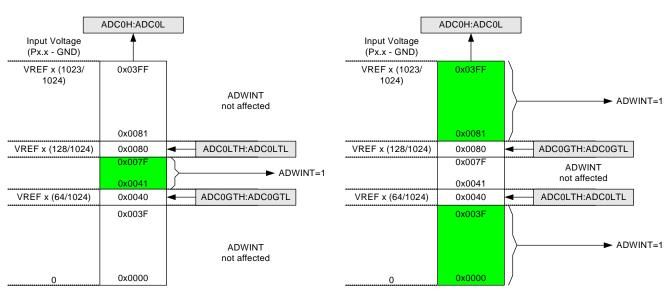
Figure 14.6. ADC Window Compare Example: Right-Justified Single-Ended Data
