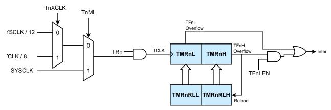
Figure 25.4. 16-Bit Mode Block Diagram
