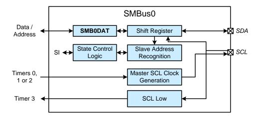
Figure 24.1. SMBus0 Block Diagram
