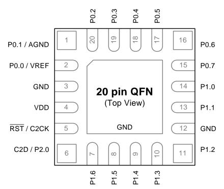
Figure 3.2. C8051F850/1/2/3/4/5-GM and C8051F850/1/2/3/4/5-IM Pinout
