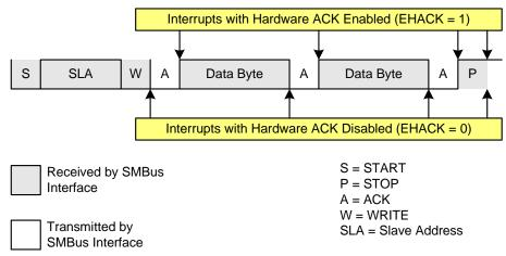
Figure 24.7. Typical Slave Write Sequence
