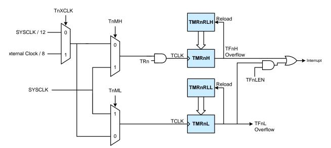
Figure 25.5. 8-Bit Mode Block Diagram
