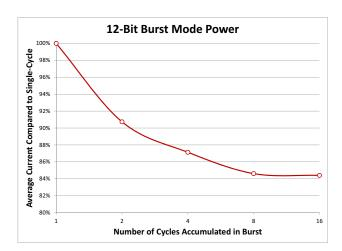
Figure 14.5. Burst Mode Accumulation Power Savings
