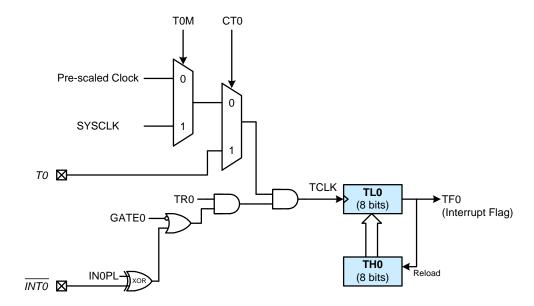
Figure 25.2. T0 Mode 2 Block Diagram
