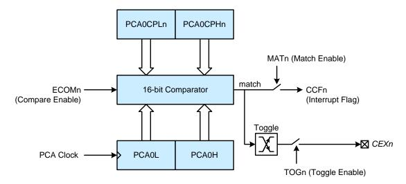
Figure 20.4. PCA High-Speed Output Mode Diagram
