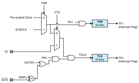
Figure 25.3. T0 Mode 3 Block Diagram
