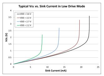
Figure 1.6. Typical V<sub>OL</sub> vs. Sink Current
