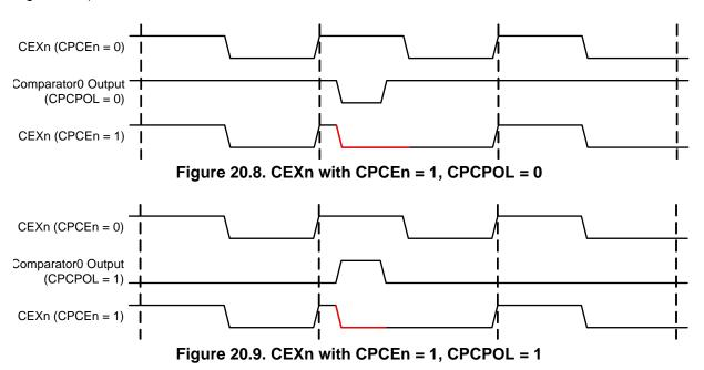
In the PWM cycle following the current cycle, should the Comparator 0 output remain logic low when CPCPOL = 0 or logic high when CPCPOL = 1, CEXn will continue to be cleared. See Figure 20.10 and Figure 20.11.
