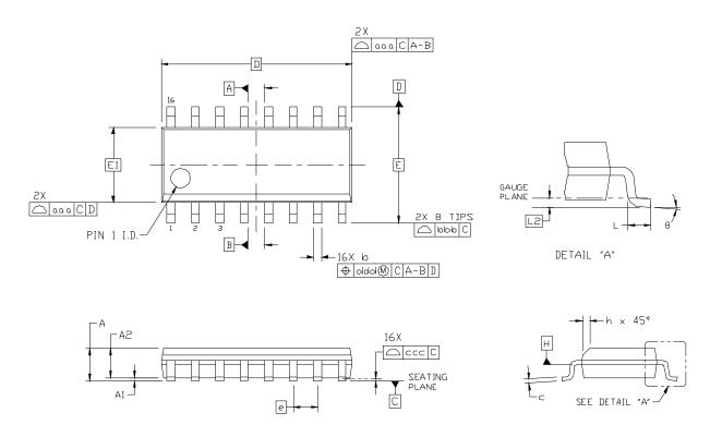
Figure 7.1. SOIC-16 Package Drawing
