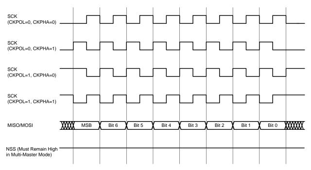
Figure 23.5. Master Mode Data/Clock Timing
