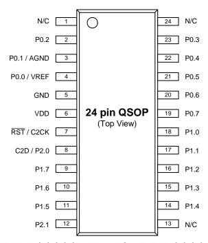
Figure 3.1. C8051F850/1/2/3/4/5-GU and C8051F850/1/2/3/4/5-IU Pinout
