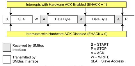
Figure 24.5. Typical Master Write Sequence
