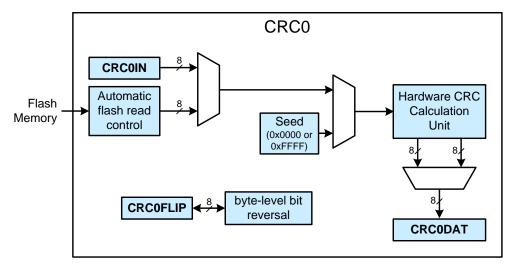
Figure 18.1. CRC0 Block Diagram
