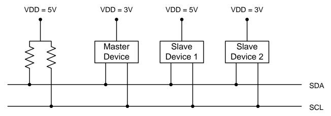
Figure 24.2. Typical SMBus Configuration
