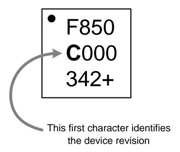
Figure 28.2. QFN-20 Package Revision Marking
