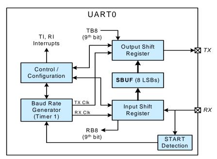
Figure 26.1. UARTO Block Diagram
