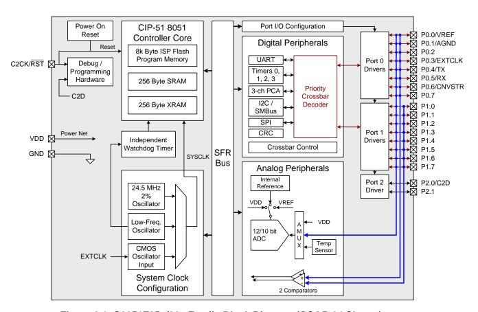
Figure 2.1. C8051F85x/86x Family Block Diagram (QSOP-24 Shown)
