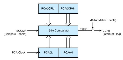
Figure 20.3. PCA Software Timer Mode Diagram
