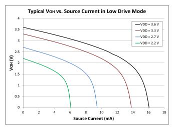
Figure 1.5. Typical  $V_{OH}$  vs. Source Current
