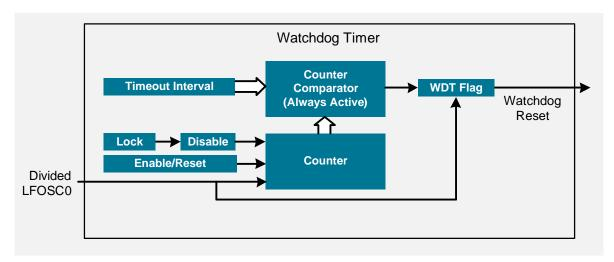
Figure 27.1. Watchdog Timer Block Diagram
