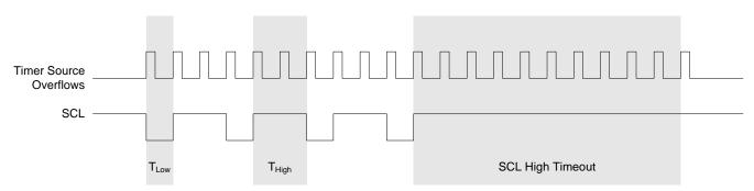
Figure 24.4. Typical SMBus SCL Generation
