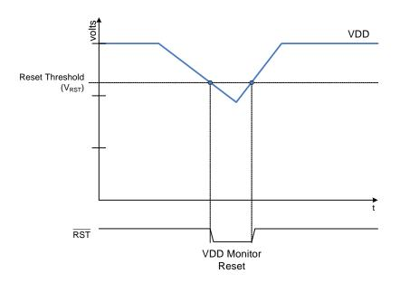
Figure 22.3. VDD Supply Monitor Threshold
