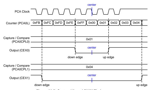
Figure 20.7. Center-Aligned PWM Timing
