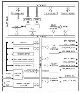
Figure 15.1. CIP-51 Block Diagram
