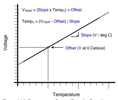
Figure 14.8. Temperature Sensor Transfer Function
