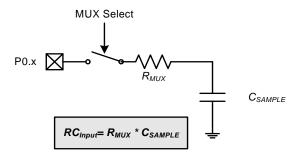
Note: The value of CSAMPLE depends on the PGA Gain. See electrical specifications for details.
