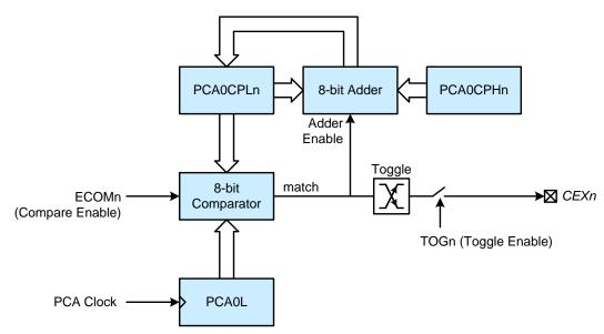
Figure 20.5. PCA Frequency Output Mode
