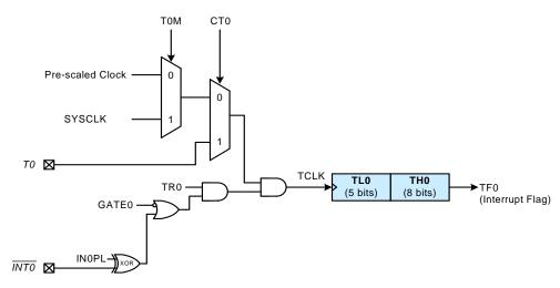
Figure 25.1. T0 Mode 0 Block Diagram
