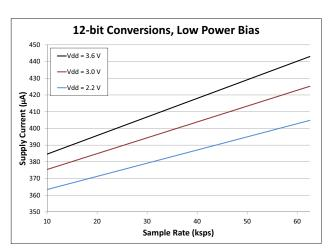
Figure 1.4. Typical ADC Power Consumption in Normal (Always-On) Mode
