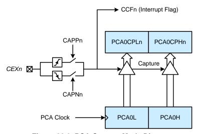
Figure 20.2. PCA Capture Mode Diagram
