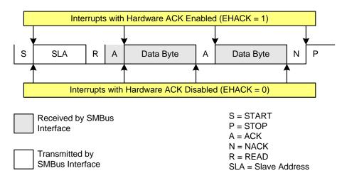
Figure 24.6. Typical Master Read Sequence
