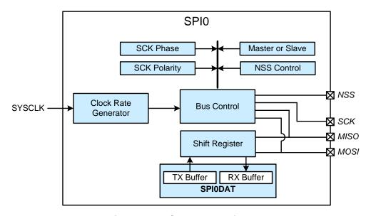
Figure 23.1. SPI0 Block Diagram
