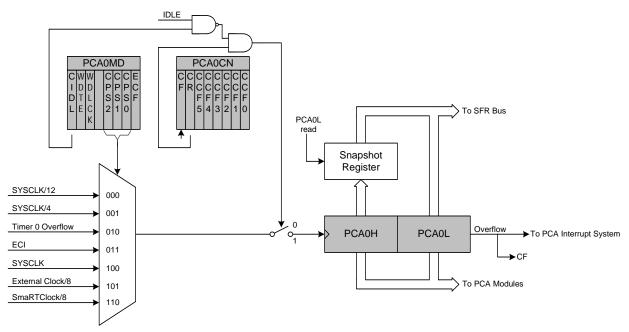
Figure 33.2. PCA Counter/Timer Block Diagram
