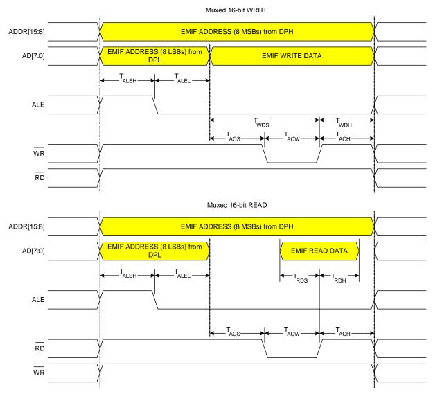
Figure 10.7. Multiplexed 16-bit MOVX Timing
