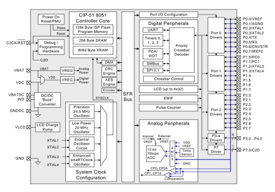
Figure 1.2. C8051F961 Block Diagram
