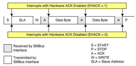
Figure 28.5. Typical Master Write Sequence
