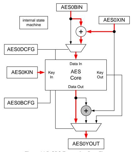
Figure 14.5. CBC Encryption Data Flow
