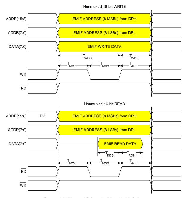
Figure 10.4. Non-multiplexed 16-bit MOVX Timing
