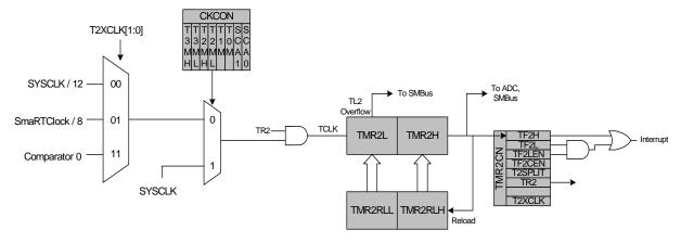
Figure 32.4. Timer 2 16-Bit Mode Block Diagram
