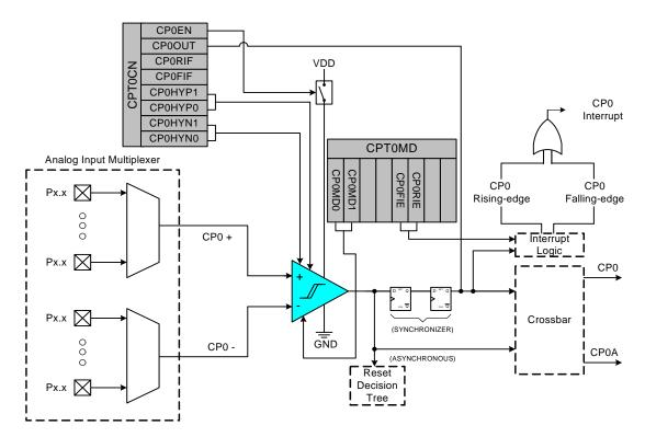
Figure 7.1. Comparator 0 Functional Block Diagram
