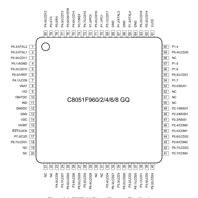
Figure 3.3. TQFP-80 Pinout Diagram (Top View)
