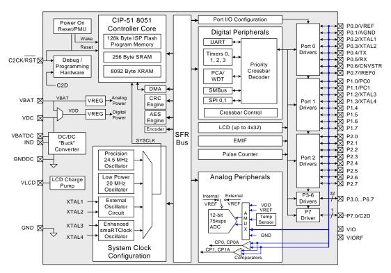
Figure 1.1. C8051F960 Block Diagram
