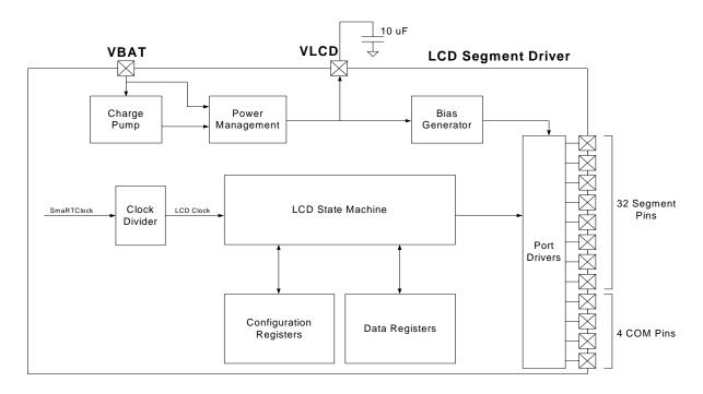
Figure 26.1. LCD Segment Driver Block Diagram
