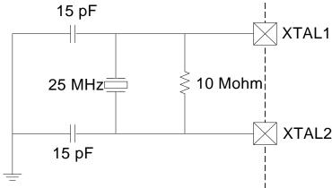
Figure 23.2. 25 MHz External Crystal Example
