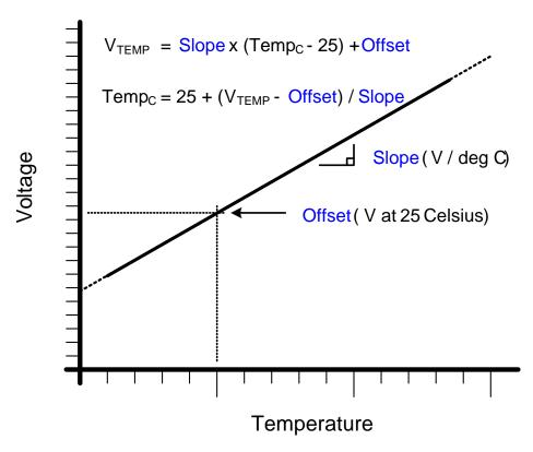
Figure 5.8. Temperature Sensor Transfer Function
