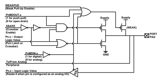
Figure 27.2. Port I/O Cell Block Diagram
