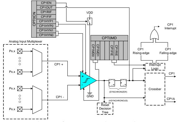
Figure 1.16. Comparator 1 Functional Block Diagram
