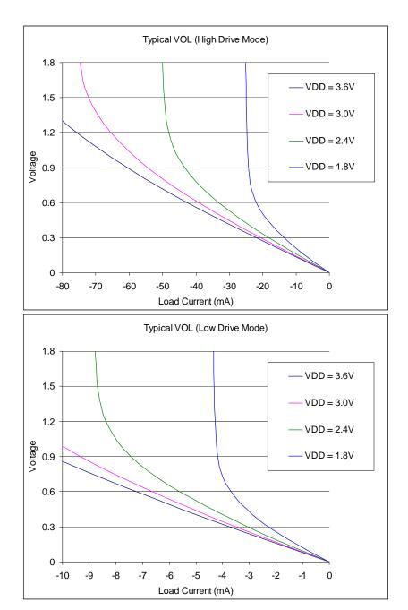
Figure 4.3. Typical VOL Curves, 1.8-3.6 V
