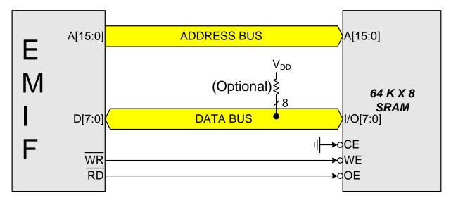
Figure 10.2. Non-multiplexed Configuration Example
