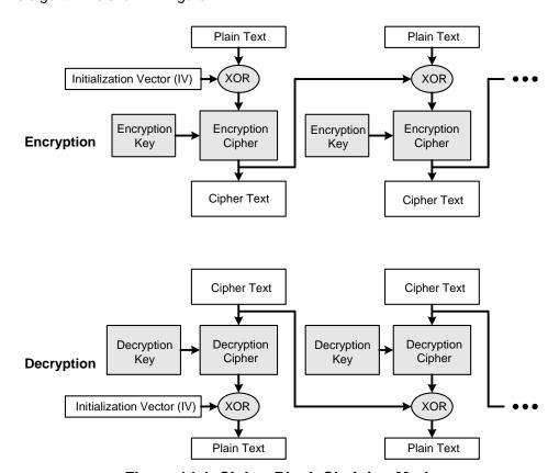
Figure 14.4. Cipher Block Chaining Mode
