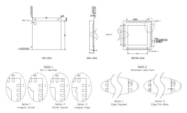
Figure 3.7. Typical QFN-40 Package Drawing
