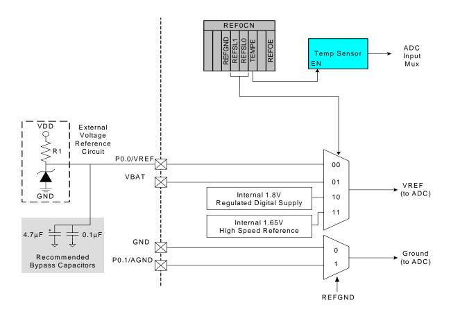
Figure 5.10. Voltage Reference Functional Block Diagram
