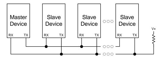
Figure 29.6. UART Multi-Processor Mode Interconnect Diagram
