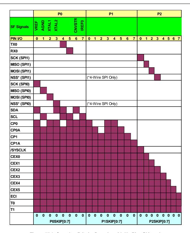
Figure 27.3. Crossbar Priority Decoder with No Pins Skipped
