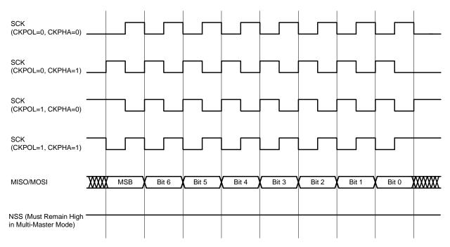
Figure 30.5. Master Mode Data/Clock Timing
