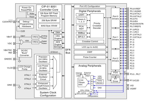
Figure 1.7. C8051F966 Block Diagram
