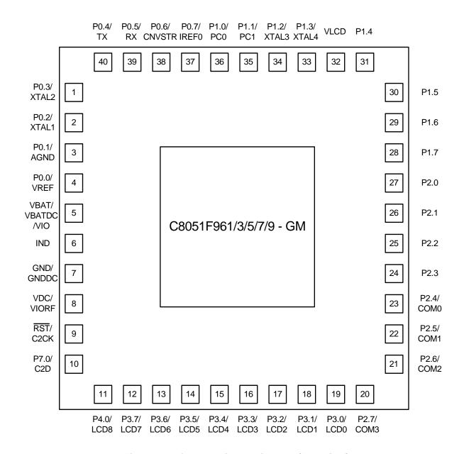
Figure 3.2. QFN-40 Pinout Diagram (Top View)
