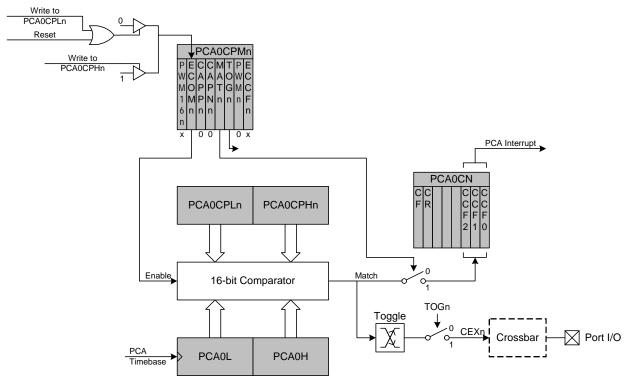
Figure 33.6. PCA High-Speed Output Mode Diagram
