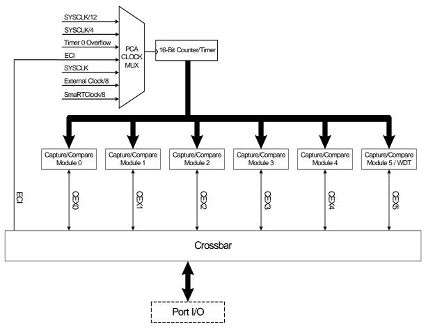
Figure 33.1. PCA Block Diagram
