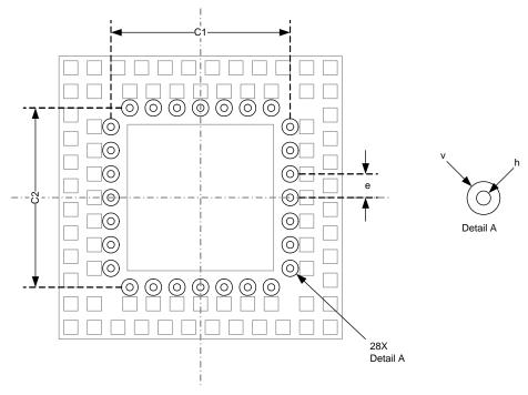
Figure 3.6. Recomended Inner Via Placement
