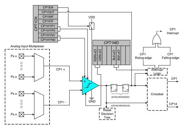
Figure 7.2. Comparator 1 Functional Block Diagram
