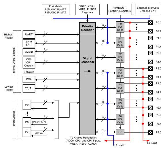
Figure 1.11. Port I/O Functional Block Diagram
