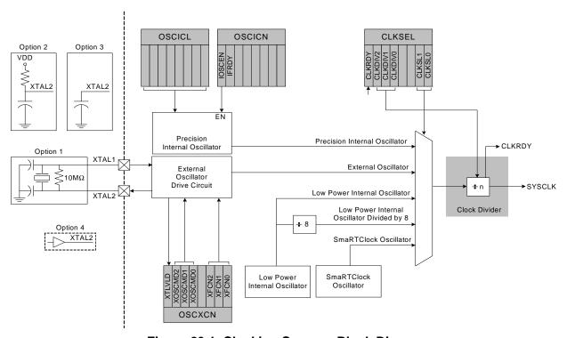
Figure 23.1. Clocking Sources Block Diagram
