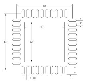
Figure 3.8. QFN-40 Landing Diagram
