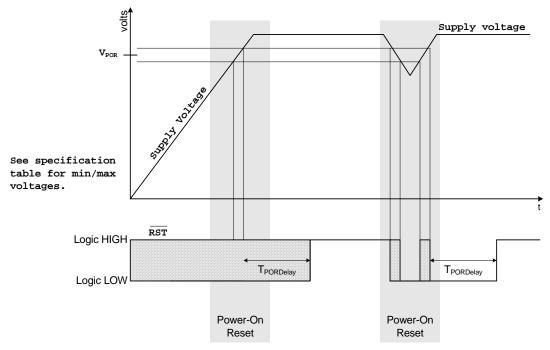
Figure 22.2. Power-On Reset Timing Diagram
