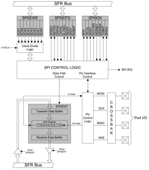
Figure 31.1. SPI Block Diagram
