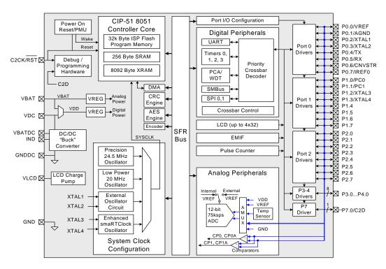
Figure 1.8. C8051F967 Block Diagram
