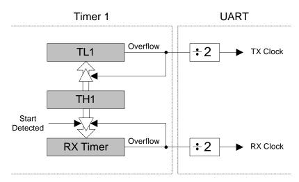
Figure 29.2. UARTO Baud Rate Logic
