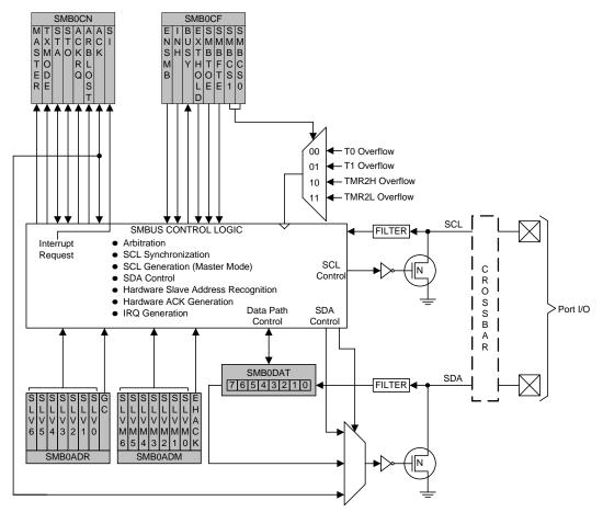
Figure 28.1. SMBus Block Diagram
