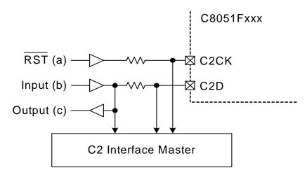
Figure 34.1. Typical C2 Pin Sharing
