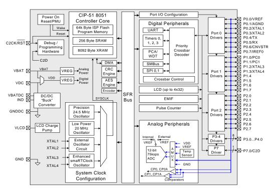
Figure 1.6. C8051F965 Block Diagram
