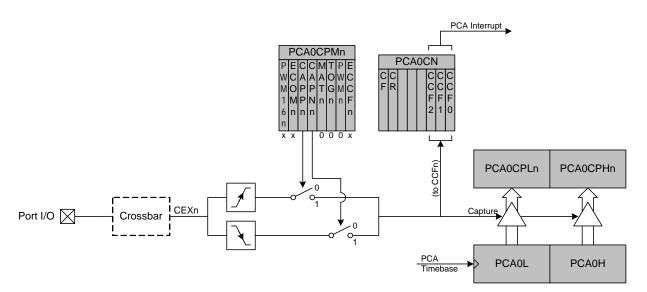
Figure 33.4. PCA Capture Mode Diagram
