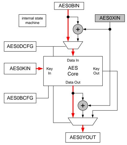
Figure 14.3. AES Block Cipher Data Flow
