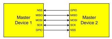
Figure 30.2. Multiple-Master Mode Connection Diagram
