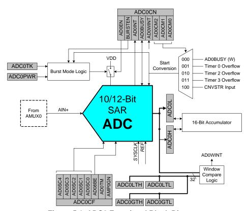
Figure 5.1. ADC0 Functional Block Diagram
