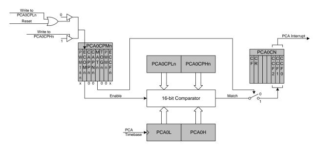
Figure 33.5. PCA Software Timer Mode Diagram
