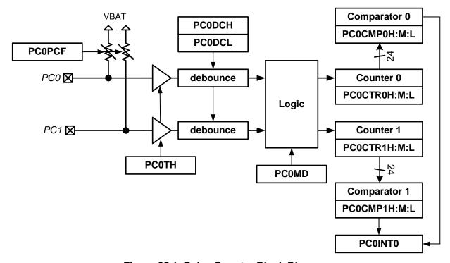
Figure 25.1. Pulse Counter Block Diagram
