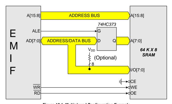
Figure 10.1. Multiplexed Configuration Example
