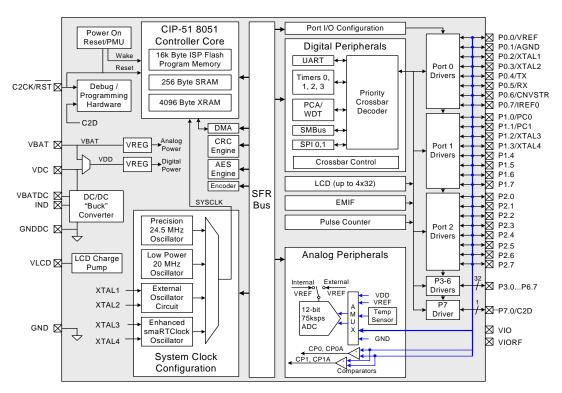
Figure 1.9. C8051F968 Block Diagram
