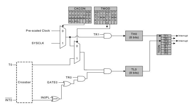
Figure 32.3. T0 Mode 3 Block Diagram
