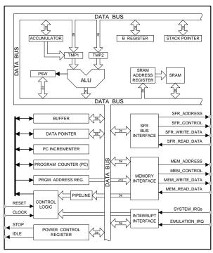
Figure 8.1. CIP-51 Block Diagram
