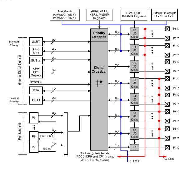
Figure 27.1. Port I/O Functional Block Diagram
