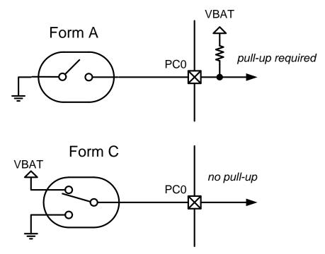
Figure 25.3. Reed Switch Configurations
