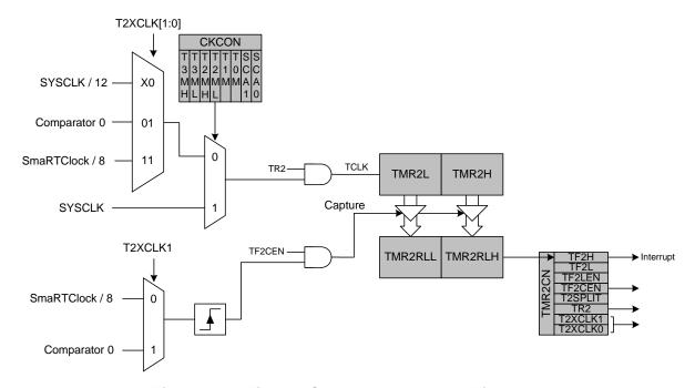
Figure 32.6. Timer 2 Capture Mode Block Diagram
