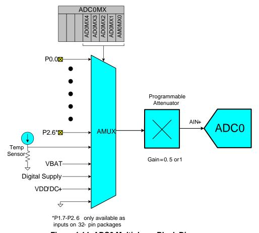
Figure 1.14. ADC0 Multiplexer Block Diagram
