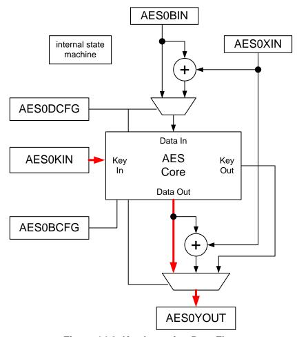
Figure 14.2. Key Inversion Data Flow
