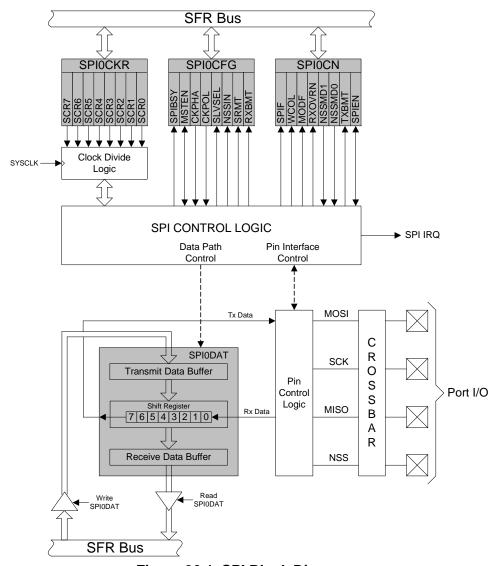
Figure 30.1. SPI Block Diagram
