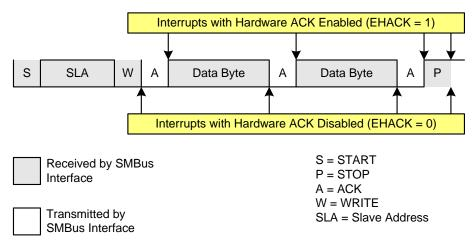
Figure 28.7. Typical Slave Write Sequence
