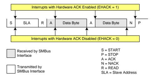
Figure 28.6. Typical Master Read Sequence
