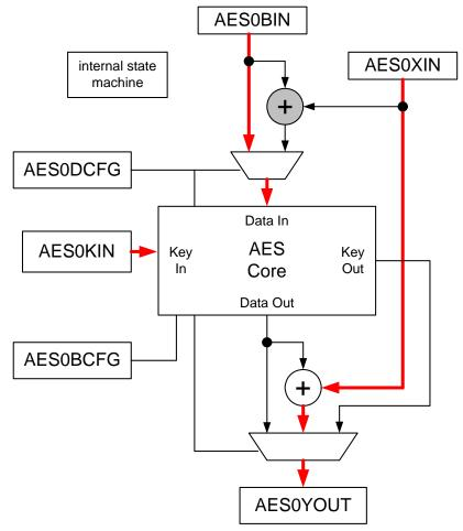
Figure 14.8. Counter Mode Data Flow
