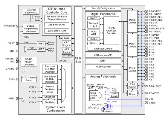
Figure 1.5. C8051F964 Block Diagram
