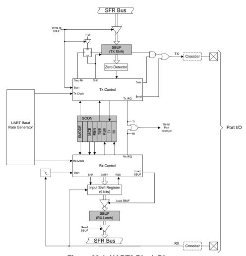
Figure 29.1. UARTO Block Diagram
