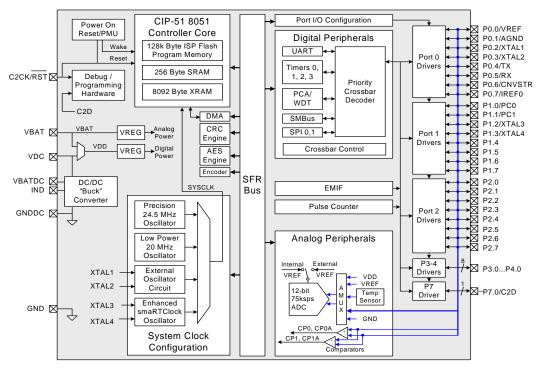
Figure 1.4. C8051F963 Block Diagram
