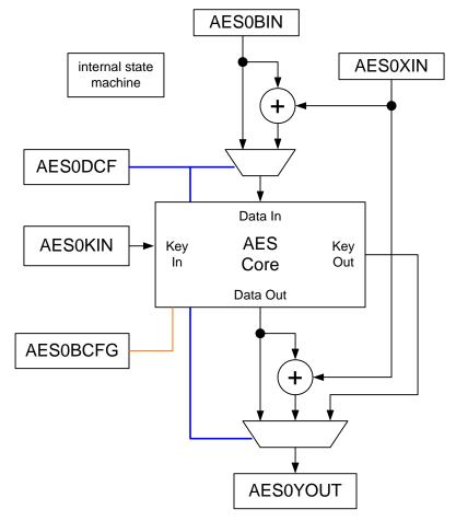
Figure 14.1. AES Peripheral Block Diagram
