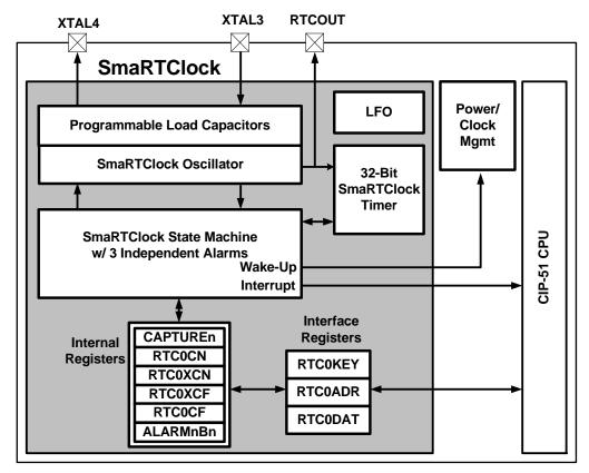
Figure 24.1. SmaRTClock Block Diagram
