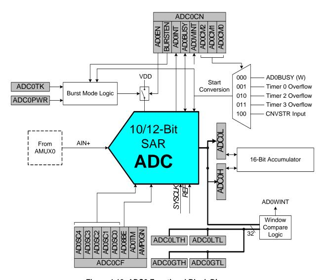
Figure 1.13. ADC0 Functional Block Diagram
