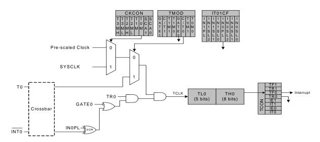
Figure 32.1. T0 Mode 0 Block Diagram
