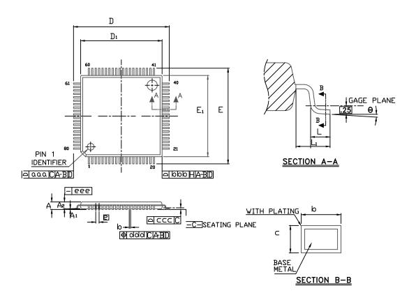
Figure 3.9. TQFP-80 Package Drawing
