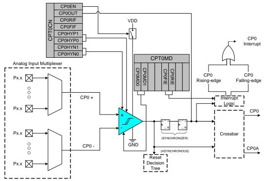
Figure 1.15. Comparator 0 Functional Block Diagram
