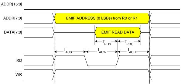
Figure 10.5. Non-multiplexed 8-bit MOVX without Bank Select Timing
