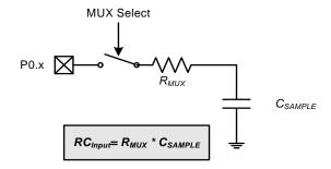
Note: The value of CSAMPLE depends on the PGA Gain. See Table 4.12 for details.
