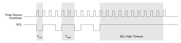
Figure 28.4. Typical SMBus SCL Generation
