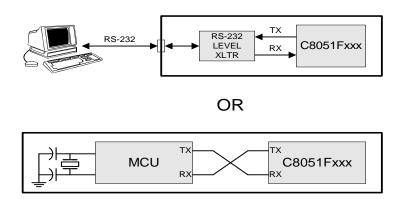
Figure 29.3. UART Interconnect Diagram
