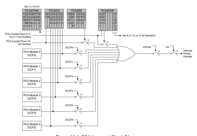
Figure 33.3. PCA Interrupt Block Diagram
