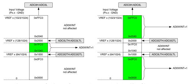
Figure 5.6. ADC Window Compare Example: Left-Justified Single-Ended Data
