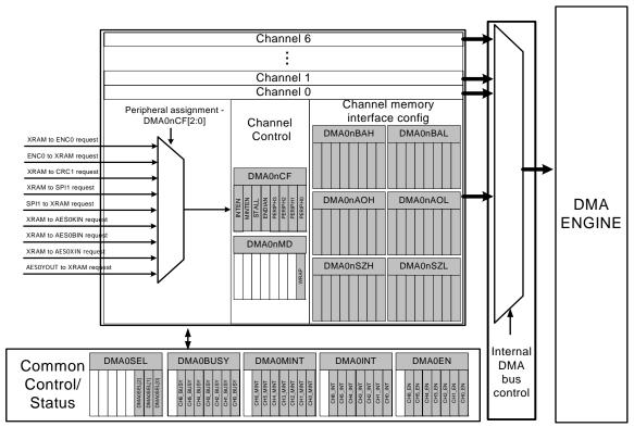
Figure 11.1. DMA0 Block Diagram
