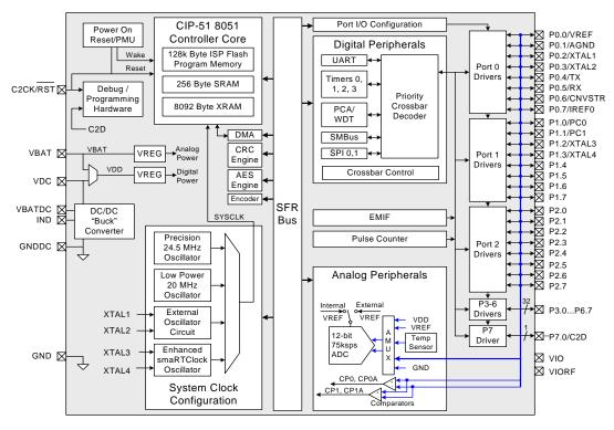
Figure 1.3. C8051F962 Block Diagram
