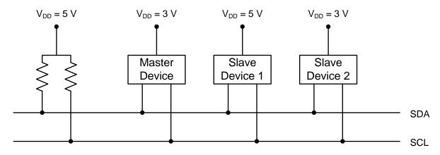
Figure 28.2. Typical SMBus Configuration
