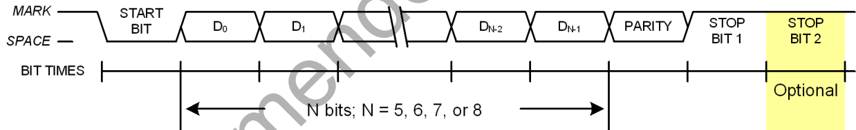
Figure 26.3. UART1 Timing With Parity
