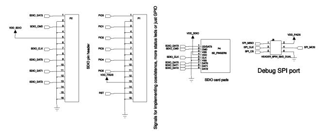
A number of programmable bi-directional input/outputs (I/O) are provided on a number of pads on the board, arranged for a surface mounted pin header that can be soldered on if needed. PIO[0:5] are powered from VDD\_PADS.
