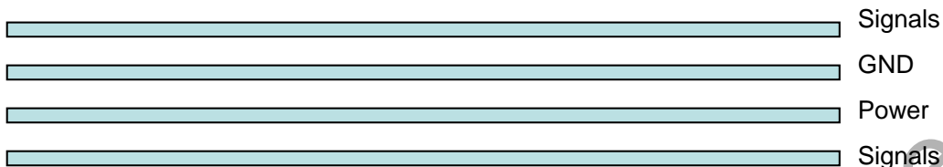
Figure 29: Typical 4-layer PCB construction
