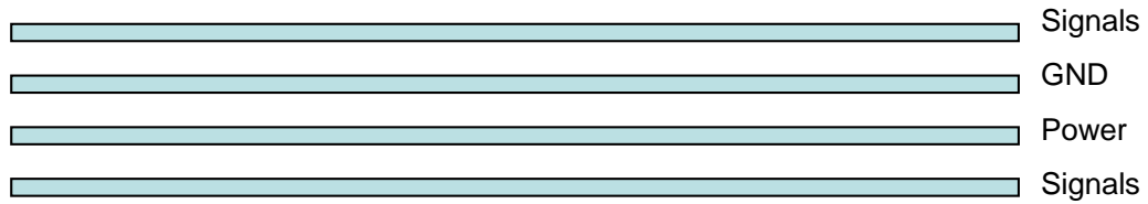
Figure 17: Typical 4-layer PCB construction
