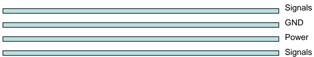
Figure 8: Typical 4-layer PCB construction
