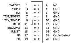
Table 9.3. Debug connector pinout
