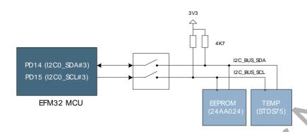
The EEPROM device consists of 256 bytes (256 x 8) and has a lifetime of 1,000,000 erase/write cycles. The EEPROM's I<sup>2</sup>C address is 0xA0.
