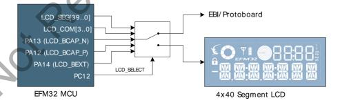
When the LCD\_SELECT signal is enabled, a 22nF capacitor is connected between LCD\_BCAP\_N and LCD\_BCAP\_P, and a 1uF capacitor is connected between LCD\_BEXT and GND. This allows the use of the internal voltage booster to power the LCD if desired.
