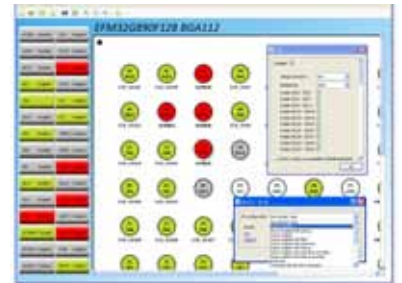
energyAware Designer Fast and easy EFM32 MCU configuration tool that instantly resolves pin conflicts.
