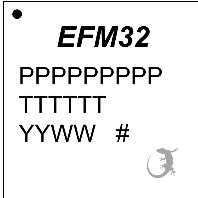
Figure 7.3. QFN48 Package Marking
