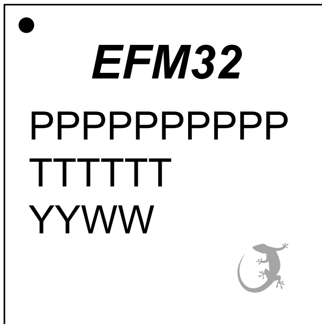
Figure 10.3. TQFP48 Package Marking
