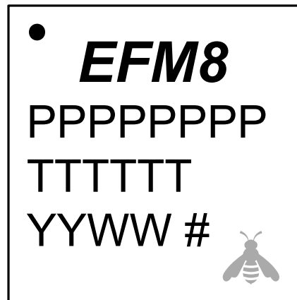
Figure 7.3. QFN28 Package Marking
