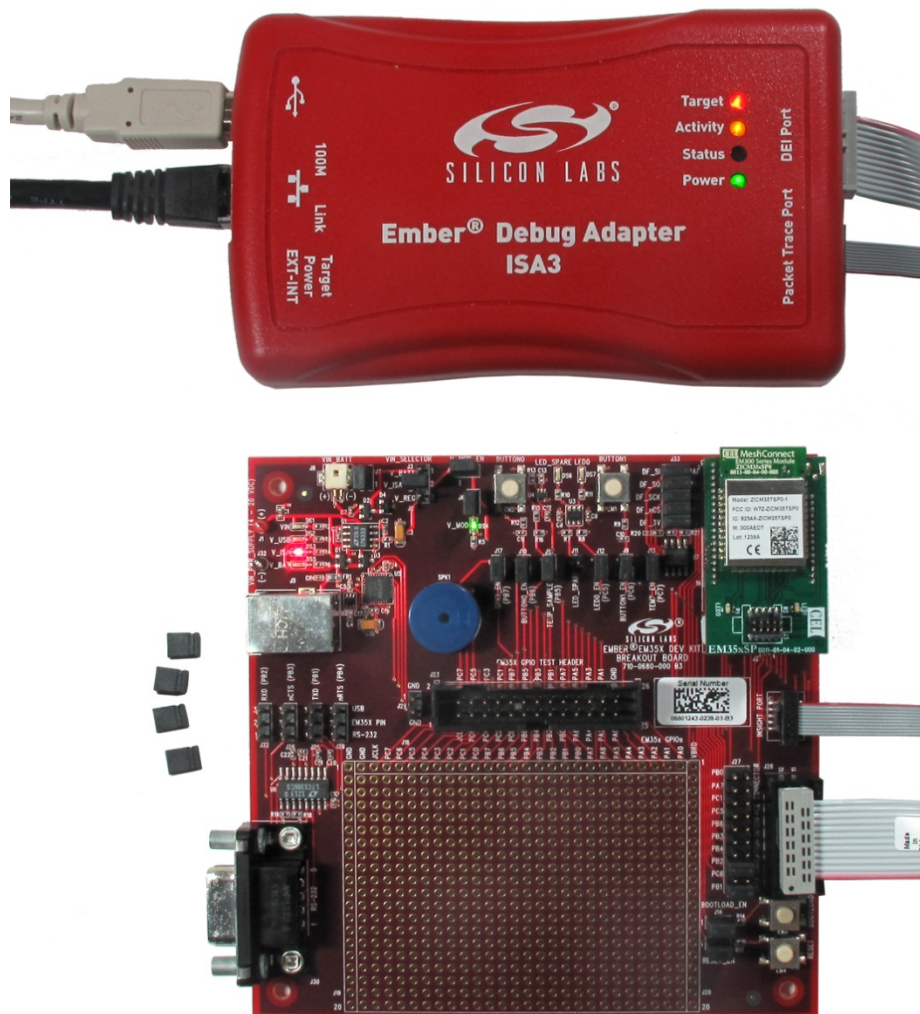
Figure 12. Ember Debug Adapter (ISA3) Supplying Power; Pass-through UART Being Used for Serial Communication
