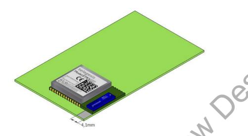
Figure 12. Adding a no copper / no component area
