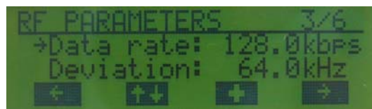
Figure 8. Menu Page: RF Parameters 3/6 (Modulation is 2GFSK)
