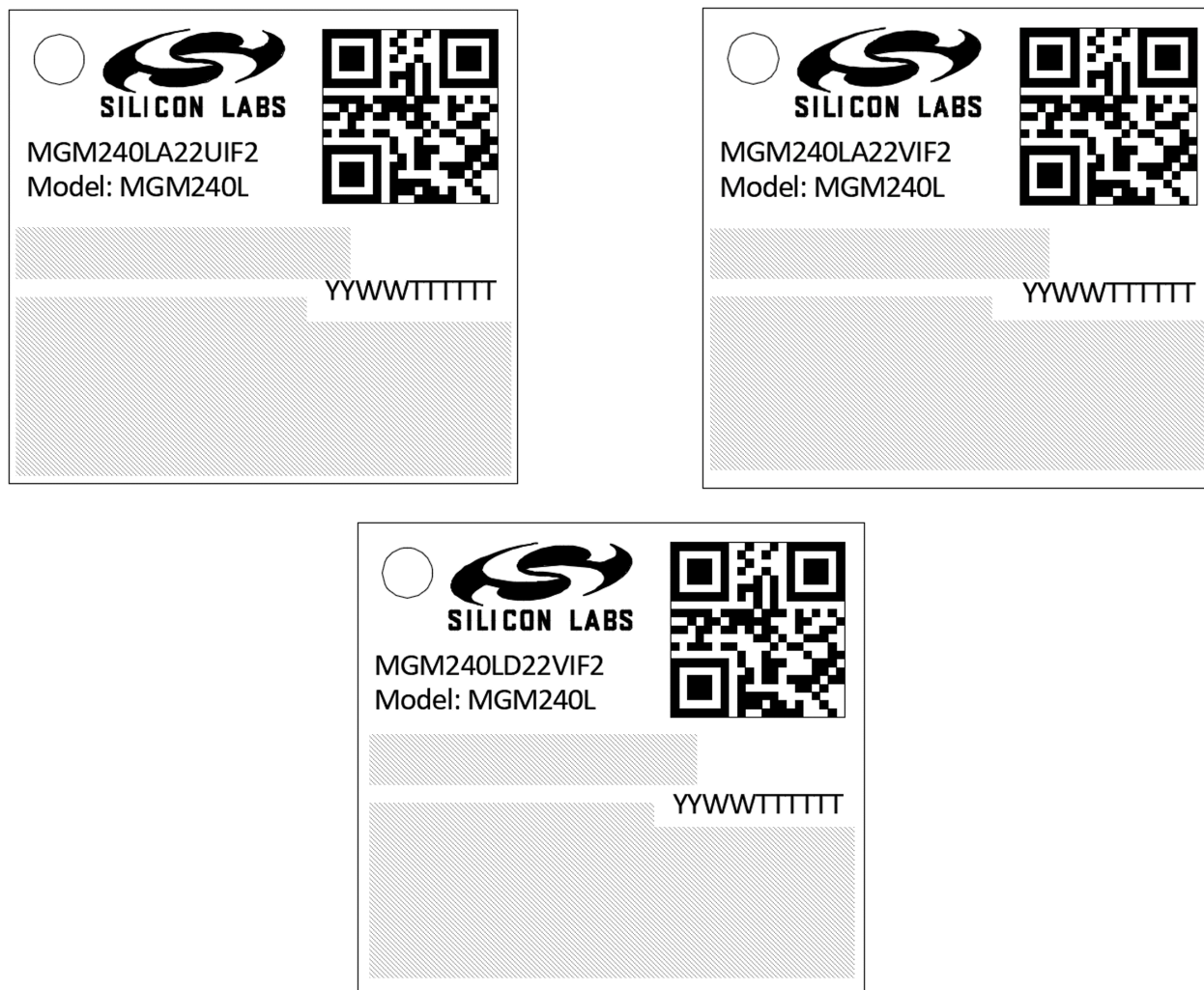
Figure 8.4. MGM240L Top Marking
