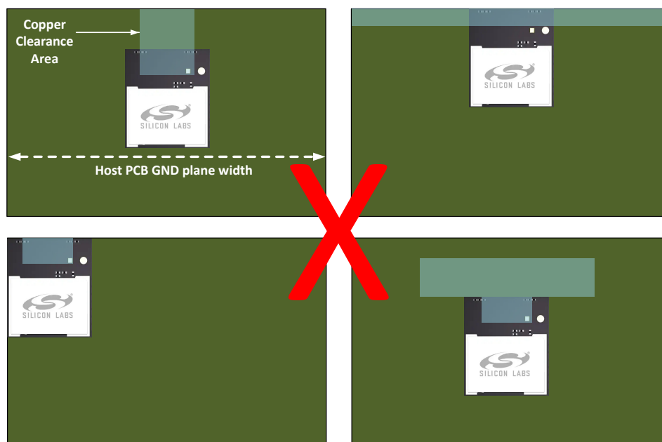
Figure 7.3. Non-Optimal Layout Examples
