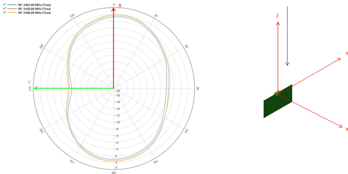
Figure 4.3. Typical 2D Antenna Radiation Patterns - Theta 90° (Front View) Gain (dBi)
