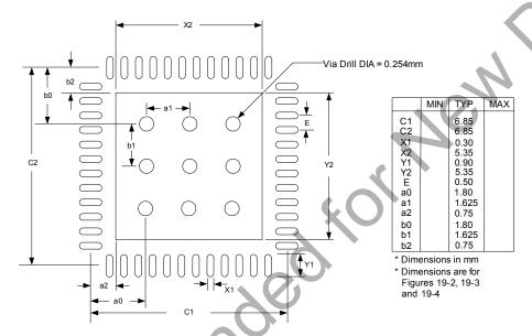
Figure 6.3. PCB Footprint for the EM358x
