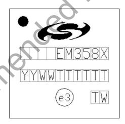
Figure 6.7. Part Marking for EM358x
