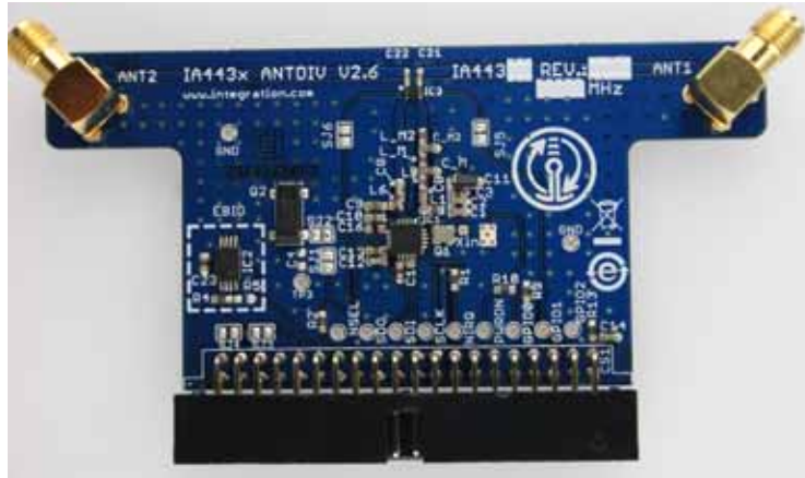
Figure 15. Antenna Diversity Testcard (May be Ordered Separately)
