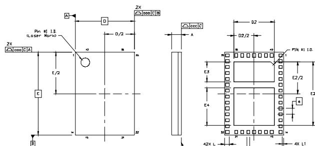
42-Pin QFN/LGA Package Diagram Dimensions
