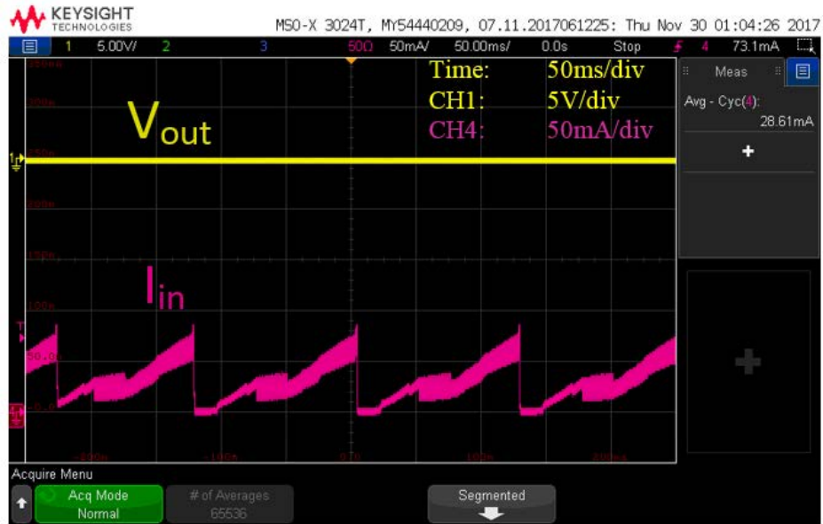
Figure 9.1. Si3406 Non-Isolated Flyback EVB Output Voltage and Input Current when the Output is Shorted
