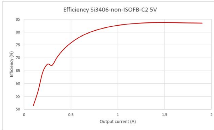
Figure 3.1. Si3406 Non-Isolated Flyback EVB Overall Efficiency (50 V Input, 5 V Output, Class 2 PD)
